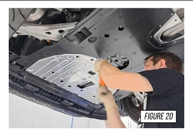
Make your final adjustments to the tips to ensure they are in a position you like. Once the desired positioning is achieved work from the front of the car to the back, tightening all the clamps fully and ensuring there is proper clearance of the chassis, and braces.
