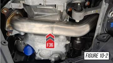
With your AWE front pipe (**F36**) installed, take a moment to verify that it sits centered above the heat shield as shown in **Figure 11**.
