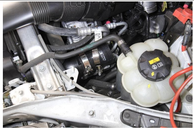
9. Install the reducer coupler along with provided T-bolt clamps onto the intercooler outlet. *Do not tighten any of the clamps yet because the coupler will need to be adjusted later when the HPS pipe is installed.
