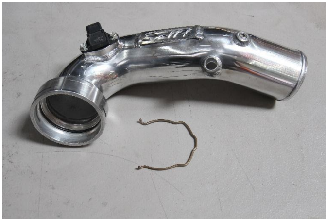
8. Install and secure the air temp sensor onto the HPS charge pipe using the provided M6-12mm bolts, then insert the O-ring into the quick connect.
