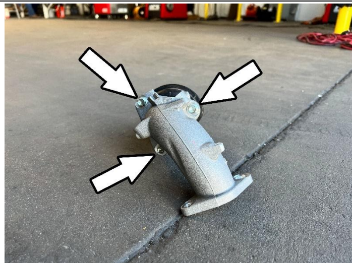
13. Remove the three 10mm bolts securing the resonator from the turbo outlet elbow.
