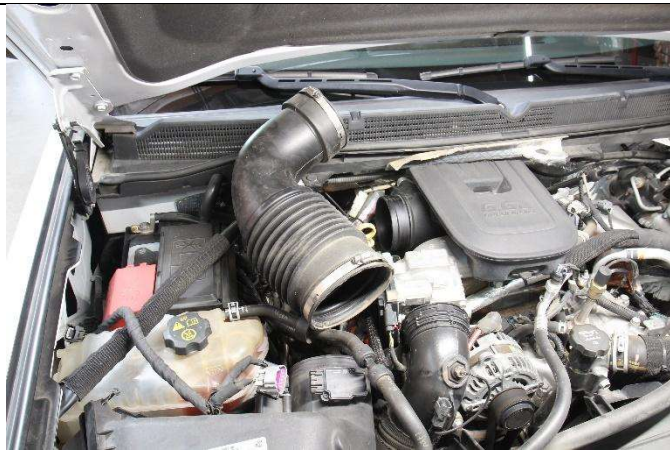
4. Remove the factory intake hose from the vehicle.
