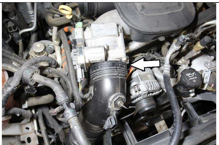
11. Using a flat head screwdriver, rotate the locking mechanism counterclockwise to release the charge pipe from the throttle body.
