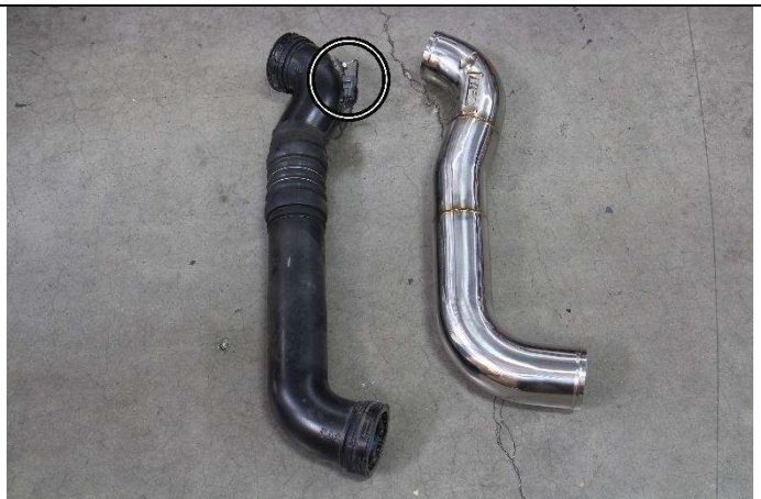
13. Remove the temperature sensor from the factory charge pipe to the HPS charge pipe.
