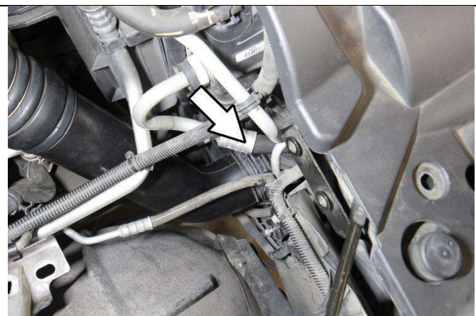
10. Using a flat head screwdriver, rotate the locking mechanism counterclockwise to release the charge pipe from the intercooler.
