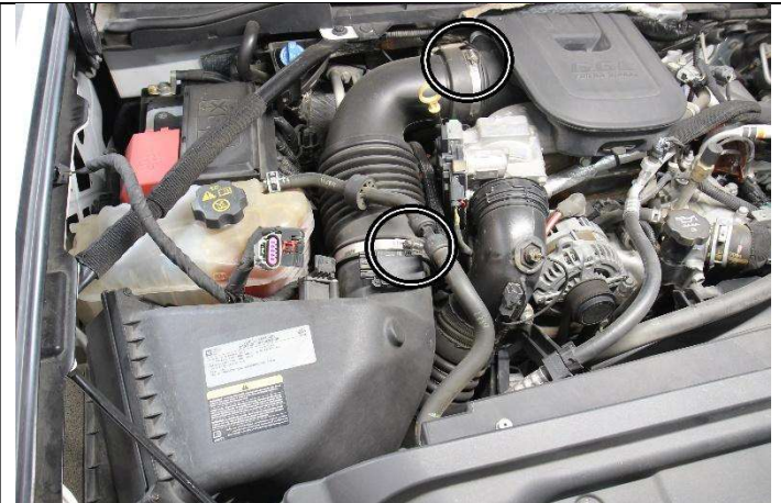
3. Loosen the hose clamp securing the factory hose from the air box and the turbo inlet.
