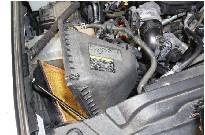
6. Remove the upper air box assembly from the vehicle.
