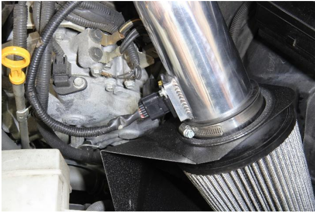
22. Re-connect the passenger and driver side MAF sensor harness connector onto the MAF sensor.
