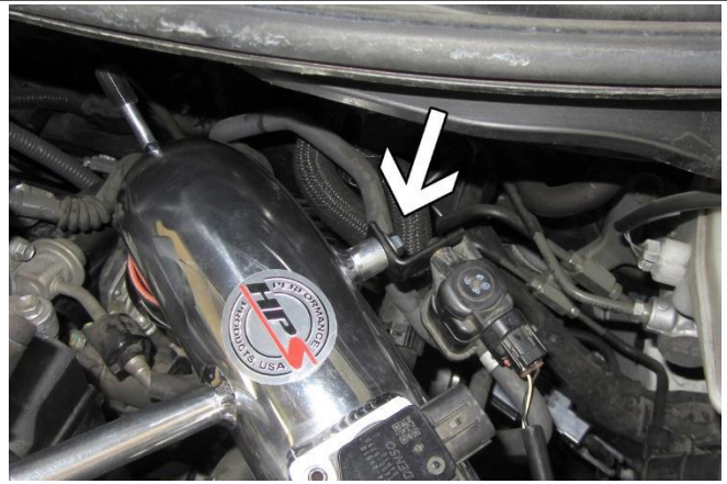
17. Insert the HPS intake pipe into the coupler, but do not secure the intake bracket or the T-bolt clamp at this time. Install the sensor bracket onto the pipe using a M6x12mm bolt and washer.
