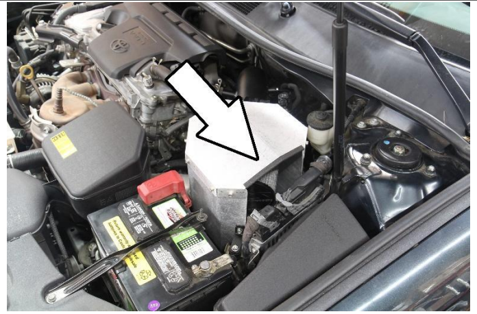
23. Install the heat shield lid onto the heat shield using the provided three M5x12mm bolt, then install the thin edge trim onto the area shown.
