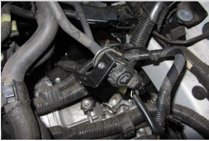
16. Install and secure the "L" bracket onto the evap. sensor reusing the factory screw.
