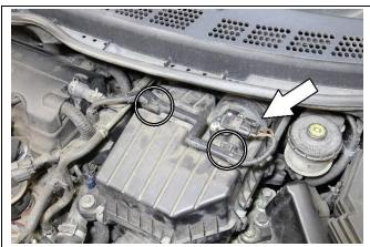
2. Depress the retaining clips securing the mass air flow sensor electrical harness, then disconnect the MAF sensor harness connector.
