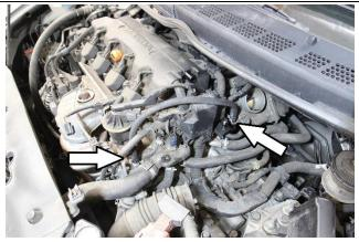
9. Install and secure the 8mm EPDM hose along with the provided FIC clamps onto the coolant hose barbs replacing the factory hose removed in the last step.
