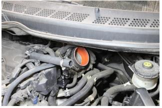
11. Insert the reducer coupler along with the provided T-bolt clamps onto the throttle body.
