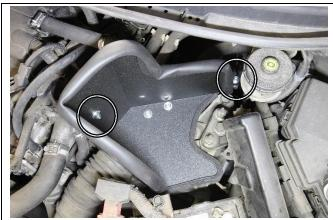
18. Secure the flat bracket onto the factory heatshield bracket using the provided M6x12mm bolt and washer.
