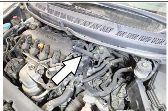
10. Install and secure the 16mm EPDM hose along with the provided EMSC clamps onto the breather barb.
