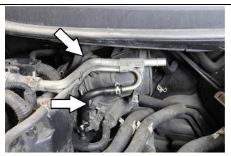
7. Disconnect any electrical harnesses from the intake hose. Loosen the hose clamp securing the intake hose and remove it from the vehicle.
