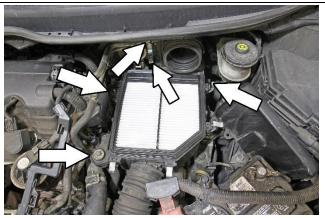
5. Remove the two 10mm bolts securing the lower air box assembly. Loosen the hose clamp securing the air intake hose, then depress the hose clamp securing the breather pipe from the intake hose. Remove the factory air duct hose from the lower air box assembly.
