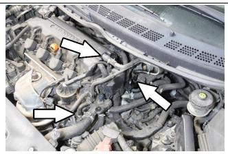
8. Loosen the hose clamps securing the breather hose from the valve cover. Using a pair of pliers, loosen the factory coolant hose clamps securing the coolant hose from the throttle body and the lower hose assembly. \* Use a small bag to catch any residual coolant. Remove the coolant hose and breather hose assembly from the vehicle.
