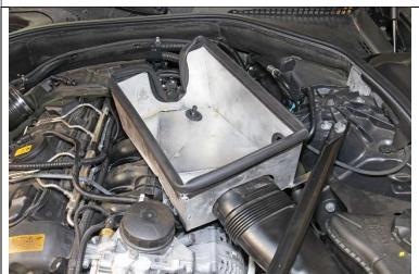
14. Insert the heat shield into the vehicle.
