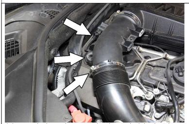
4. Loosen the hose clamp securing the stock air intake tube. Disconnect the mass air flow sensor harness connector and carefully lift the stock air intake tube from its grommet.
