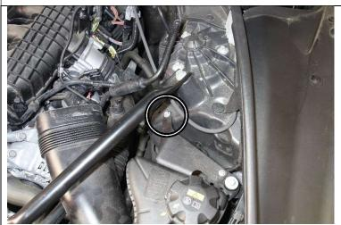
12. Remove the 10mm bolt securing the coolant reservoir shown in the image above.
