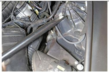
13. Insert the provided 1" vibration mount replacing the 10mm bolt removed in step 12.
