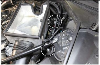
15. Align and secure the heat shield bracket onto the vibration mount using the provided M6 nut. Re-attach the rubber harness mounts onto the bracket.
