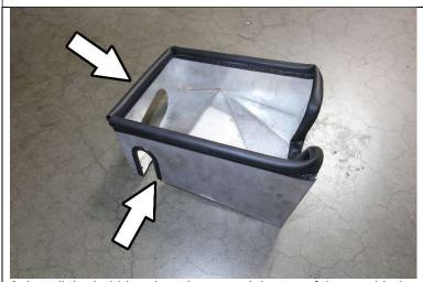
8. Install the bubble edge trim around the top of the provided HPS heatshield. Install the thin edge trim into the cutout shown in the image above.
