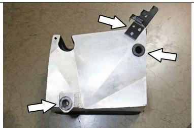
10. Install the factory rubber grommet into the bracket of the heat shield. Insert the provided rubber grommet into the slot located near the bracket. Install and secure the factory mounting bracket using the provided M4 bolts.
