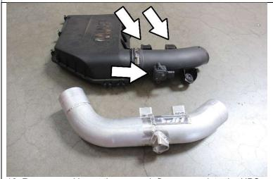
16. Remove and insert the mass air flow sensor into the HPS intake pipe using the provided M4 allen bolts. Insert the factory engine cover mounts into the HPS intake pipe.
