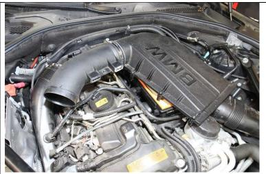
5. Remove the air intake tube along with the upper air box assembly from the vehicle.
