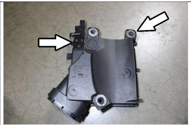
9. Remove the factory bracket and the rubber grommet mount from the lower air box assembly.
