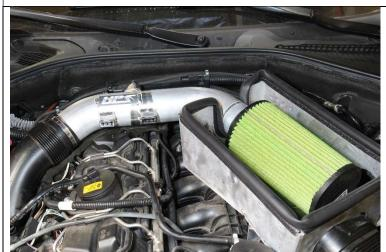
18. Insert and secure the HPS intake pipe into the vehicle. Re connect the MAF sensor harness connector.
