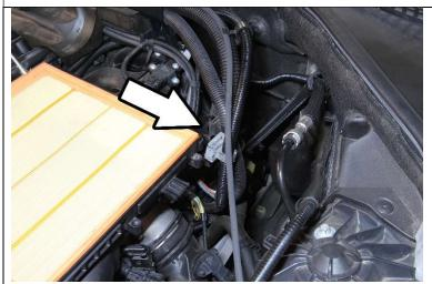
6. Disconnect the three rubber harness mounts from the lower air box assembly.
