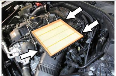
7. Lift the lower air box assembly from its grommets, then disconnect the lower air box from the air duct. Remove the lower air box assembly from the vehicle.
