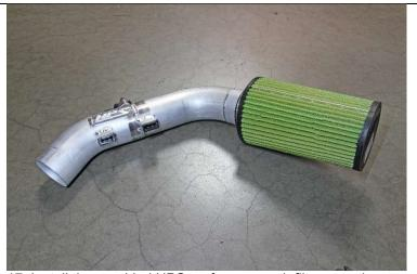
17. Install the provided HPS performance air filter onto the intake pipe.
