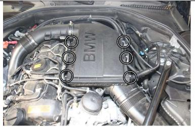
3. Loosen the six torx bolts securing the upper air box assembly.
