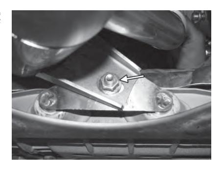
140) Tighten the downturn to downpipe 11mm V-band clamp.
