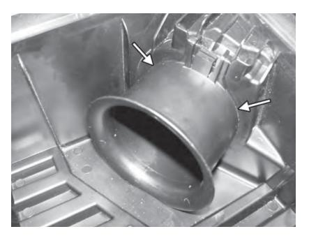
149) Apply some two part epoxy adhesive to the bottom tabs of the air straightener, and reinstall the straightener. Then, apply epoxy to permanantly attach the straightener to the airbox lid. Also apply epoxy to the top clip of the straightener.
