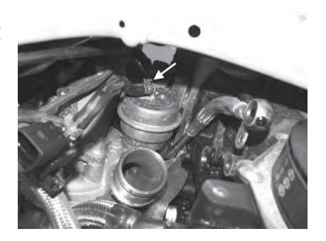
60) Remove the two T30 Torx screws that connect the compressor inlet pipe to the turbocharger.
