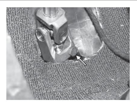
157) Making sure the steering linkage is splined into the steering rack, reinstall the 13mm bolt in the linkage and torque to 15lb-ft, then tighten an additional 90°.
