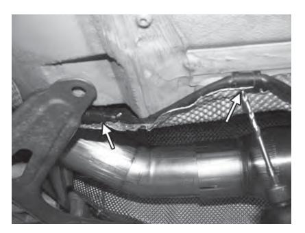
137) Route the wiring harness from the secondary air sensor over to the connector on the extension cable and connect it. It will be necessary to create a "pocket" behind the heat shield for the electrical connection to sit in to allow the exhaust cross brace mount correctly. Finally, drill a small hole in the heat shield next to the plastic grommet that is on the oxygen sensor wire.
