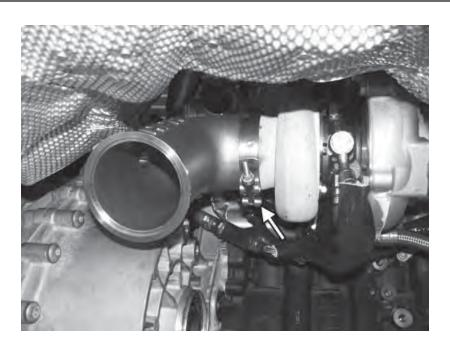
93) Install the APR downturn onto the turbocharger. Orient the V-band clamp so that the screw faces straight back towards the firewall, and is parallel to the ground. Tighten the clamp so that the downturn can still be rotated, but will not move on its own.
