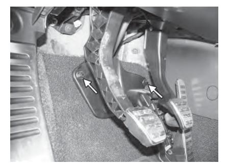
158) Install the steering linkage cover and reinstall the two 10mm bolts.
