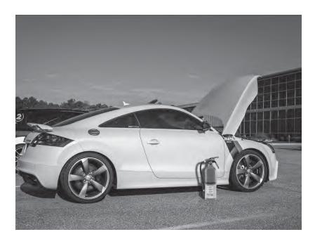
173) Start the vehicle and move it outside to a well ventilated area. Let the car warm up very slowly the first time, so as to break in the turbo blanket. The blanket will smoke very heavily for the first several times the car is run. Do NOT drive the car very hard until the smoke has subsided some. Keep an eye on the blanket to make sure it is just smoking, and is not on fire. It is normal for the blanket to continue to smoke for several heat cycles of the engine.
