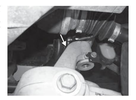
20) Lower the subframe a few more inches, and unclip the wiring harness. Also, carefully bend the steering rack heat shield up to access the clips and electrical connectors.
