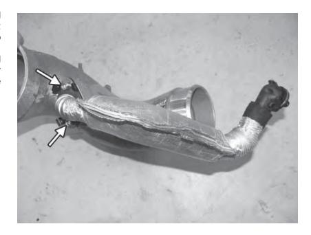
112) Install the compressor inlet pipe onto the turbocharger from underneath. As the pipe is being put into place, connect the electrical connecter to the N75 valve. Being very careful with the N75 valve ports and electrical connector so as to not break them, seat the compressor inlet into its final position. Finally, loosely install the two 6mm allen bolts.
