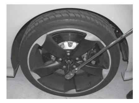
2) Remove both front wheels and remove the center cap. Reinstall the wheels and put the car on the ground. Break loose the 24mm 12-point axle bolt. Raise the car again and remove the wheels.
