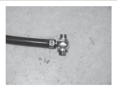
89) Remove the banjo fitting from the side of the wastegate. Install 50" of the supplied silicone hose to the fitting and crimp in place.
