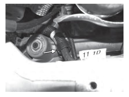
130) Reconnect the steering rack wiring harness to the existing factory clip to prevent it from moving. Be sure to bend the factory heat shield back down over the connectors.
