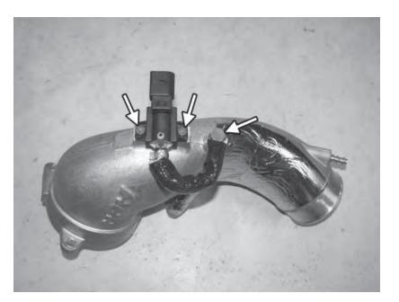
109) Using the two original T25 screws, install the N75 valve to the APR compressor inlet pipe as shown. Attach the banjo fitting to the port on the inlet hose with a crush washer on both sides of the banjo fitting, rotating the hose if necessary on the N75 valve. Once oriented correctly, crimp the hose clamp where the hose connects to the N75 valve.
