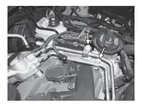
116) Reinstall the upper and lower fuel lines to the high pressure fuel pump. Hold the 14mm brass fitting to the lower line and tighten the nut with a 17mm wrench. Finally, hold the brass fitting on the upper line with a 14mm wrench and tighten the nut with a 15mm wrench.
