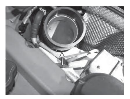
113) Make sure the compressor inlet pipe is spaced evenly away from the turbocharger heat shield. If necessary, rotate the compressor inlet pipe foward or back on the slotted mounting holes. When correctly spaced, tighten the two 6mm allen screws on the compressor inlet pipe.
