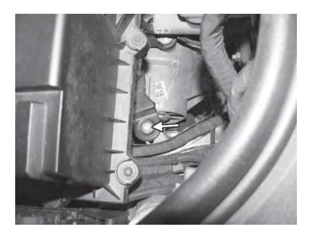
153) Install the 10mm bolt into the back of the stock airbox.
