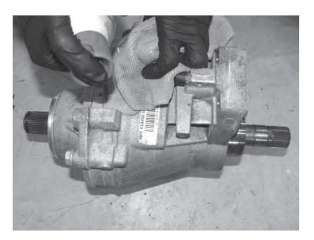
85) Clean the top of the transfer case with brake parts cleaner or some other solvent that does not leave a residue. Remove any stickers from the top of the transfer case.
