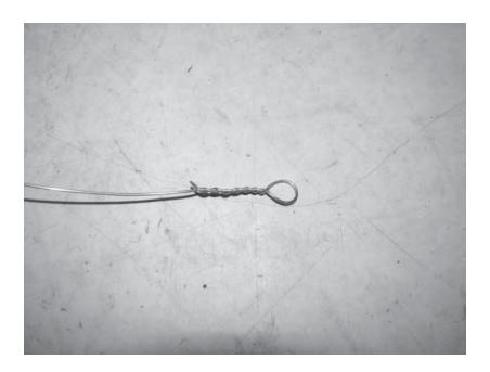
96) Put the loop on one of the hooks on the turbo blanket, and then wrap the wire in a figure eight pattern between the two adjacent hooks. Once the connection is sufficently connected, wrap the excess wire around itself to secure it.
