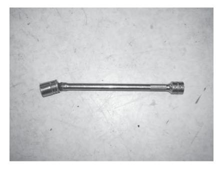
102) Tighten the upper bolt closest to the engine block using a regular 16mm socket with an extension with a wobble end.
