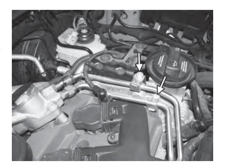
56) Remove the two 10mm triple square bolts from the fuel pump and lift up on the pump to remove it from the car.
