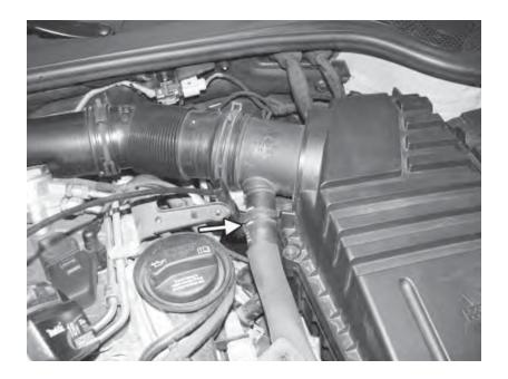
48) Remove the two T30 Torx screws that connects the stock inlet pipe to the back of the engine. Also remove the spring clamp that connects the inlet pipe to the stock compressor inlet pipe.
