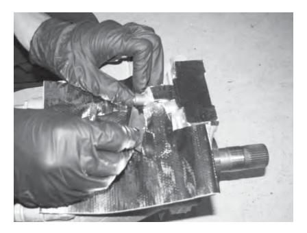
86) Before peeling off the adhesive backing, carefully place and trim the supplied gold heat shielding to the transfer case. Cut small pieces that can overlap each other to cover most of the transfer case top.
