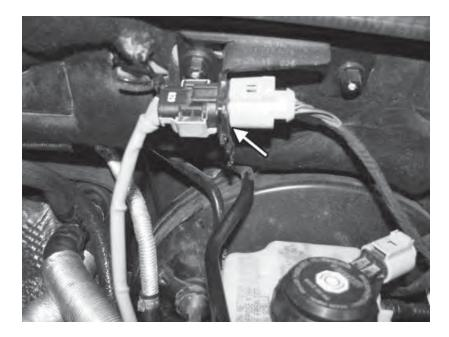
126) Reinstall the primary oxygen sensor in the side of the APR downturn. Route the wiring from the sensor up and connect it to the correct electrical connector on the firewall. Finally, clip the connector in the stock location on the firewall.
