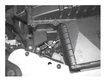
45) Remove the 5mm allen screw from the side of the stock airbox. Also remove the 10mm bolt just to the left and down from the 5mm allen screw.
