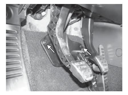
14) Remove the two 10mm bolts from the panel under the driver's footwell.
