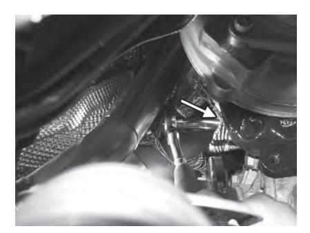
141) Tighten the downturn to turbo V-band clamp.
