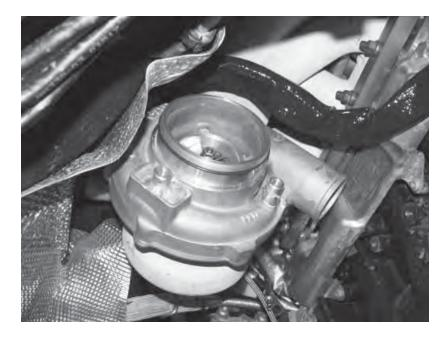
74) Install the o-ring on the turbocharger compressor, being sure not to get the o-ring twisted when installing it.
