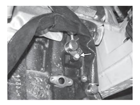
80) Connect the other end of the coolant return line to the front side of the turbocharger. Install the supplied 19mm banjo bolt with a crush washer on both sides of the banjo fitting.
