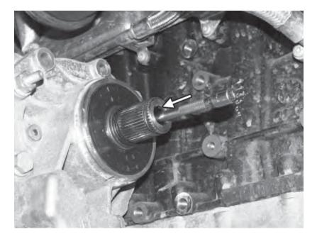
34) Using a long 1/4" extension, remove the 6mm allen bolt that is located inside the right axle stub.
