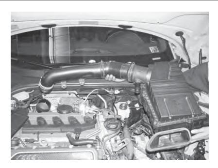
49) Remove the entire airbox and intake assembly. The airbox will come out of the car with the mounting bracket that holds it in place.
