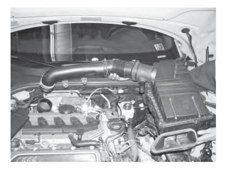
150) Reinstall the airbox and intake assembly in the car, making sure the airbox snaps into the two factory mounting posts.
