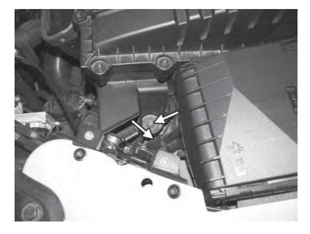
154) Install the 5mm allen screw into the side of the stock airbox. Install the 10mm bolt into the airbox mounting bracket.
