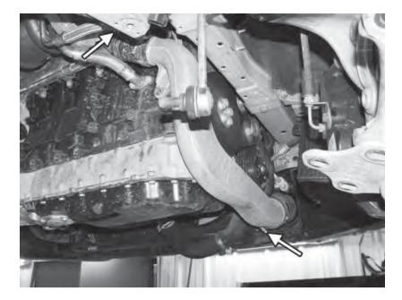
38) Loosen the 7mm hose clamps from the pancake pipe and remove the pancake pipe and the rubber hose connecting it to the turbocharger.
