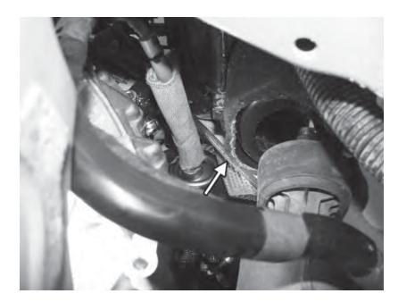
132) Remove the 10mm nut that connects the lower portion of the firewall heat shield to the firewall. Route the extension cable on the right side of the body stud so that the heat shield retains the wire with the 10mm nut reinstalled. Take care to bend back any sharp edges of the heat shield so they will not cut into the cable.
