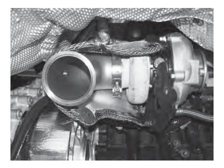
94) Wearing gloves to prevent splinters, carefully install the turbocharger blanket on the downturn and the turbine side of the turbocharger. The ring on the side of the blanket is for the primary oxygen sensor bung.
