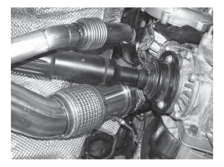
106) Install the downpipe in the car. Connect the V-band clamp to the downturn so the screw faces down and is pointed towards the front of the car. Tighten the V-band so the downpipe can still be rotated, but cannot move on its own.
