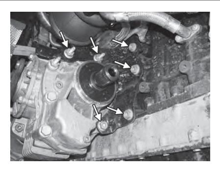
33) Remove the six 16mm bolts and nuts holding the transfer case bracket to the engine block, and remove the bracket.
