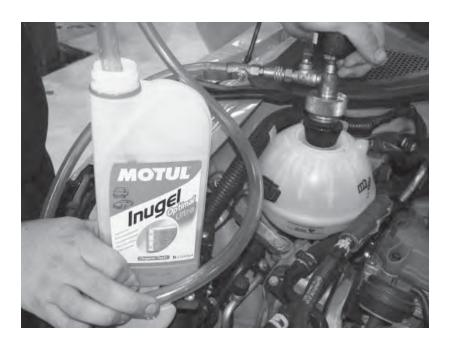
169) Using a vacuum bleeder, fill the coolant system with engine coolant.
