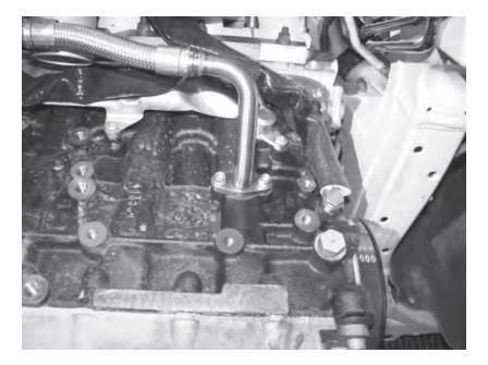
82) Install the other side of the oil drain line onto the engine block with the new supplied gasket and two 5mm allen bolts and torque the bolts to 80lb-in.
