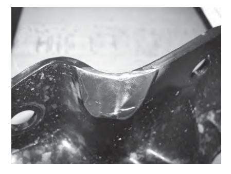
118) Using a grinder, carefully trim the corner of the transfer case brace between the two upper holes that mount it to the engine block. The APR compressor outlet hose runs very close to this, so removing some material and smoothing out any sharp edges is critical to preventing chafing on the hose.
