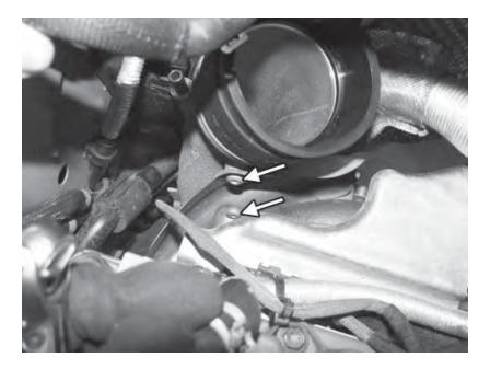
62) Remove the two T30 Torx screws that connect the compressor inlet heat shield to the compressor inlet. Remove the heat shield and then the compressor inlet pipe from the top of the car.
