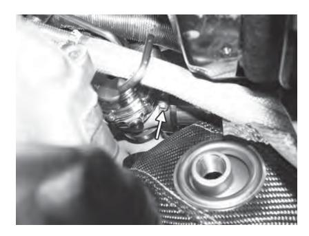
108) Take the stock N75 valve, and remove the two vacuum lines without a banjo fitting - from the top port as well as the port underneath the electrical connector. These two lines can be cut off of the N75 valve carefully with a razor blade. Finally, install some of the small heat sheathing over the remaining line.
