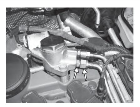
53) Loosen the lower nut on the high pressure fuel pump by holding the brass fitting in the pump with a 14mm wrench, and using a 17mm wrench to remove the nut. A rag can be used to prevent excess fuel spillage.
