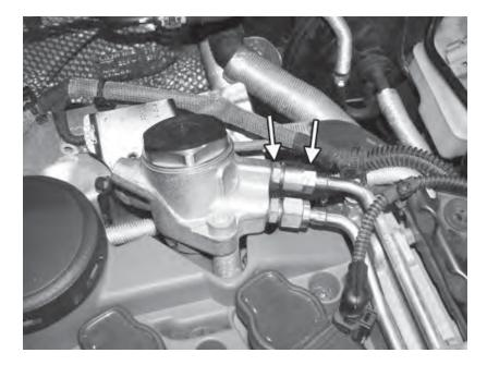
54) Loosen the upper nut on the high pressure fuel pump by holding the brass fitting in the pump with a 14mm wrench, and using a 15mm wrench to remove the nut.
