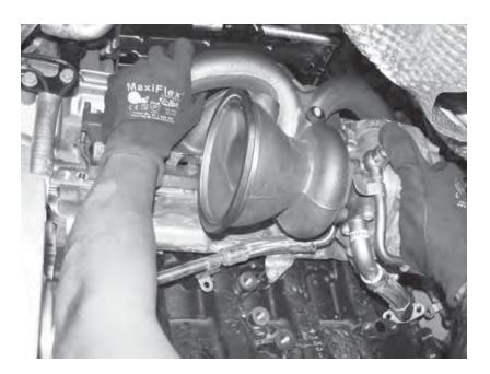
65) Lift the factory turbocharger/exhaust manifold assembly and then rotate the top side of the manifold flange away from the cylinder head. Again, do NOT loosen the lower spacers on the bottom side of the manifold. Carefully remove the assembly from the car.
