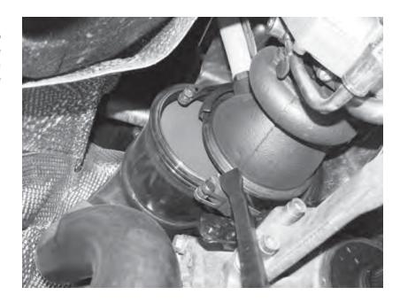
32) Remove the three 8mm allen bolts from the axle heat shield and remove from the car.
