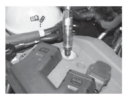
145) Remove the stock coil pack and spark plug. Gap the supplied APR spark plug to 0.024" (0.6mm). Install the APR spark plug and torque in place to 22lb-ft. Reinstall the coil packs, connect the electrical connectors, and put the two T25 screws back in place.
