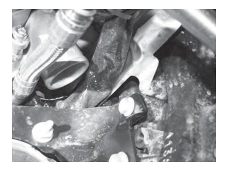
120) Install the APR compressor outlet hose and attach to the turbocharger. Do not tighten the hose clamp at the turbocharger.
