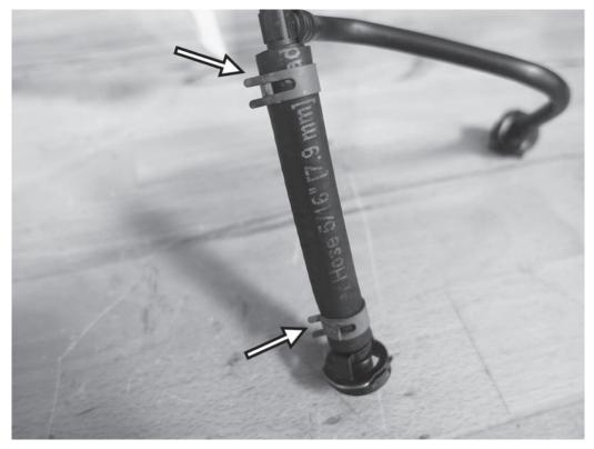
8) Install some of the supplied rubber line on the barbed fitting and secure with the supplied hose clamps. If using a tee fitting, simply install the tee in the rubber line and secure with the supplied hose clamps.
