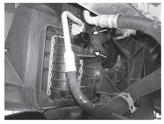
20) Once drained, disconnect the other supercharger radiator hose. On all vehicles, this is on the left side, just below the bumper beam. Remove the one T30 screw.
