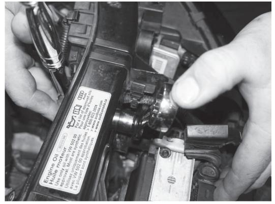
40) Using a 19mm open ended wrench on the coolant tap retainer, and a 19mm deep well socket on the coolant tap jam nut, tighten the jam nut onto the coolant tap retainer. In doing so, the coolant tap body will rotate slightly. Make sure the side port faces directly to the center of the vehicle once tightened.
