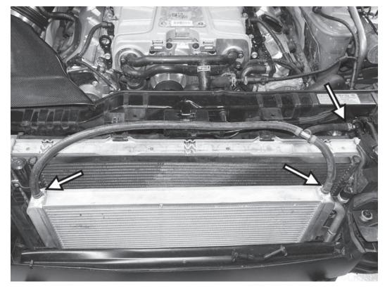
44) Connect the ends of the hose assembly to the barbs on both ends of the APR radiator, and secure with the supplied spring clamps. Connect the end off the tee fitting to the barb on the APR coolant tap and secure with a spring clamp.
