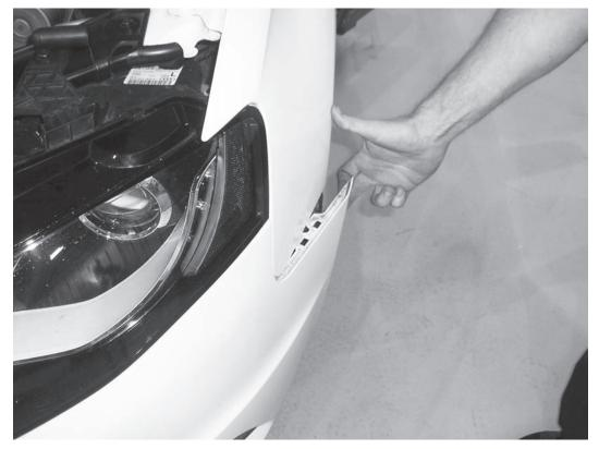
16) Carefully pull the upper corner of both sides of the bumper away from the mounting brackets on the front fenders.
