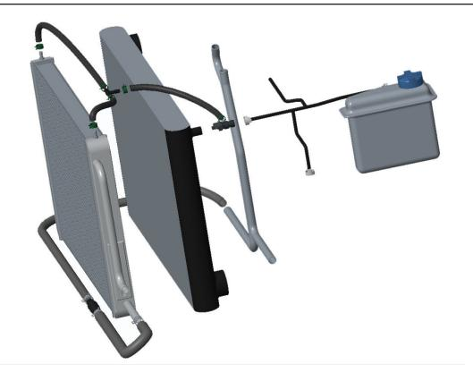
2) The recommended B8 S4/S5 is the similar to the B8.5 S4/S5. This install is covered in detail in this manual. The B8 cars have lower crossover plumbing will be needed as one of the coolant return pipes on the front of the engine is pointed towards the right side of the car. Attached the hose with the 180° bend to the lower outlet of the APR CPS radiator, and route the hose with the supplied line to the right side of the car.
