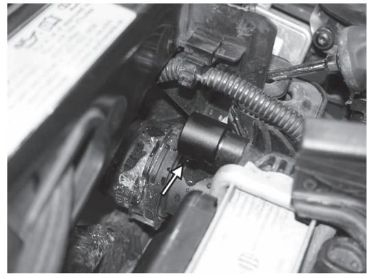
38) Install the coolant tap retainer onto the top of the coolant port on the top of the radiator. The half open side of the retainer should be facing down, with the threaded portion of the retainer facing the back of the car.
