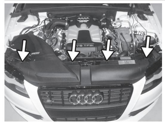
14) Remove the four T30 Torx screws from upper bumper trim cover and remove the cover.
