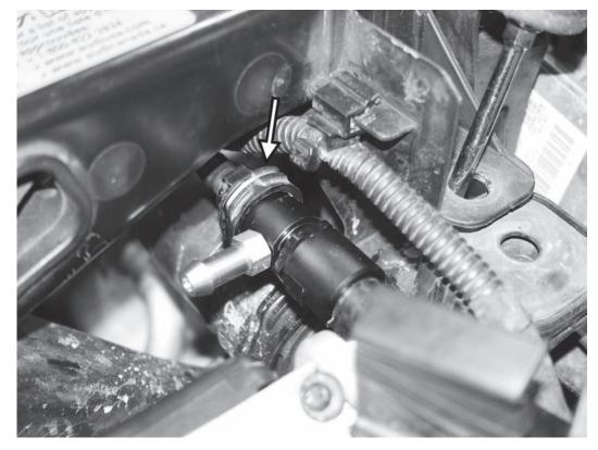
42) Reconnect the factory plastic coolant line to the back side of the APR coolant tap, making sure the clip on the fitting is locked in place.
