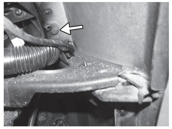
52) Pull back the fender liners on both sides and reinstall the two 10mm bolts that hold the front bumper cover to the front fender.
