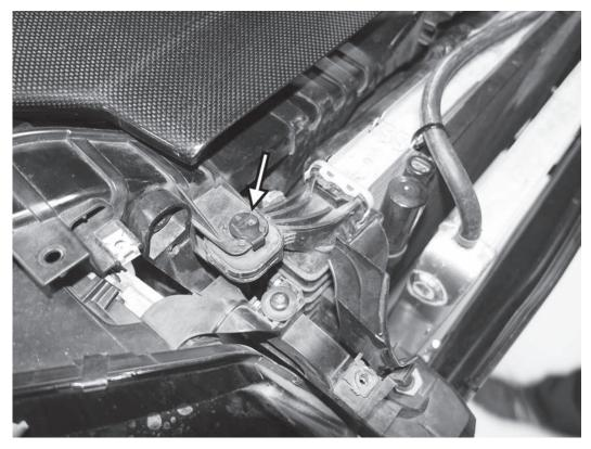
46) Push the top of the factory radiator back and install the two previously removed factory pins holding the top of the radiator to the core support.
