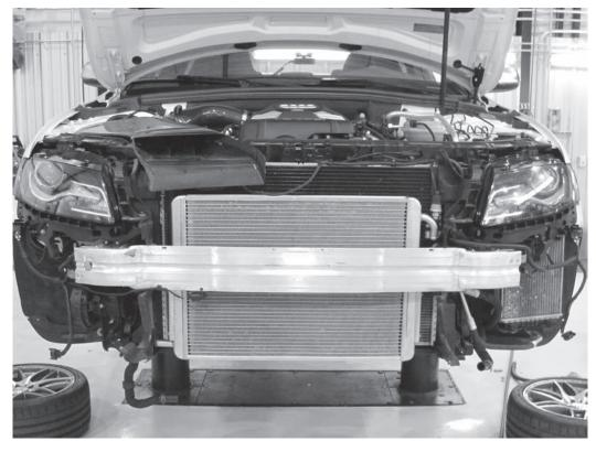
28) Attach the radiator to the bumper beam with the four factory 5mm allen bolts and lockwashers. Then, reinstall the bumper beam to the car. Be sure to reconnect the horns, the ambient air temperature sensor, and the headlight washer hose if equipped.
