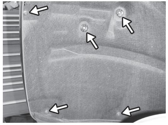
10) On both sides of the car, disconnect the three T25 Torx screws and two push tabs that hold the front half of left front fender liner to the car. Carefully bend the liner back behind the brake rotor so that it is out of the way. The B8.5 cars only have one push tab.
