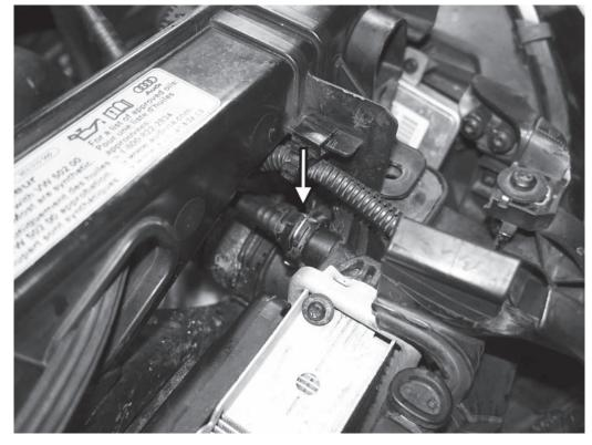
36) Carefully pull the top of the factory radiator forward. On the 3.0T's disconnect the coolant return line from the top left of the radiator by lifting up on the metal clip and then squeezing the line to disconnect. On the 4.0T's, this connection is located on the top right side of the radiator.
