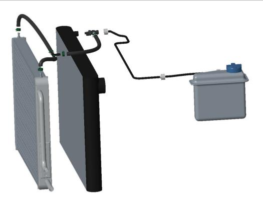
6) The S6 amd S7 4.0T has the bleeder for the engine radiator on the right side, so the bleed lines from the APR CPS radiator are routed to the right side of the car, and an APR coolant tap is used at the engine radiator.
