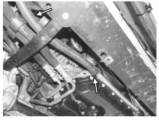
34) On the B8 only, connect the hose routed around the right side of the core support to the coolant pipe on the front of the engine, and secure with one of the medium spring hose clamps.
