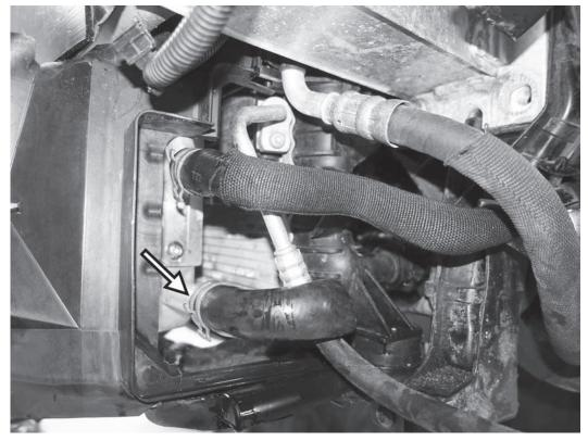
30) On a B8, connect the curved end of the supplied "J" shaped hose to the bottom inlet of the APR radiator, and secure with one of the larger spring style clamps. Route the hose behind the APR radiator and in front of the factory engine radiator.
