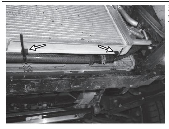
32) On the B8 only, secure the hose to the bottom lip of the APR radiator with the cable ties that have the push on retaining tabs.
