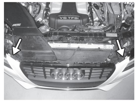
50) Reinstall the two T25 screws from the top of the bumper cover near the headlights.
