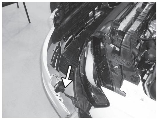
48) With an assistant, place the bumper cover near the front of the car. If equipped, reinstall the Home-Link module behind the center grille. Reconnect the left and right fog light harness. Set the bumper back to its original mounting location.
