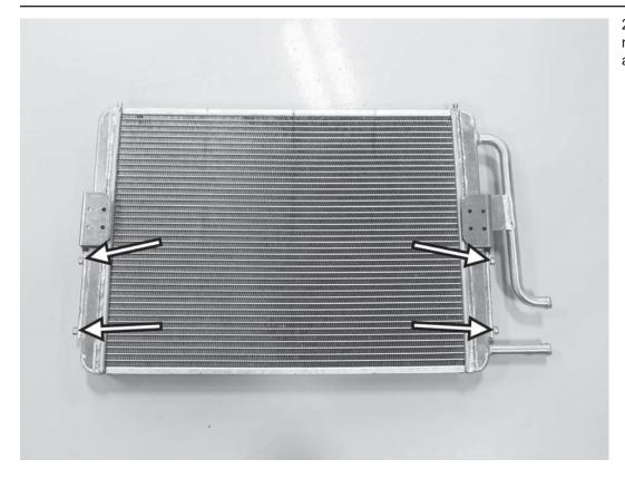
22) Temporarily bolt the radiator mounts to radiator with the four 5mm allen bolts.
