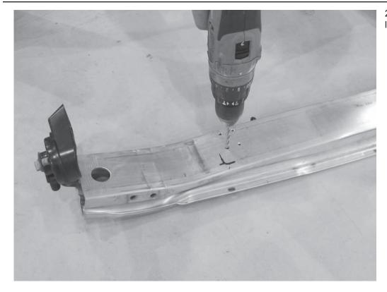
26) Drill the holes in the marked location with the supplied drill bit.
