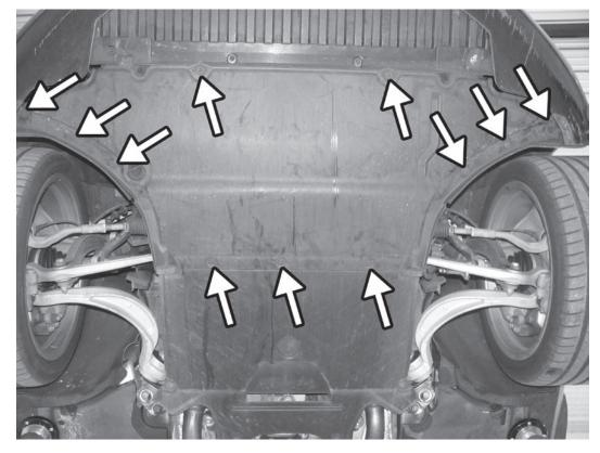
54) Reinstall the eleven quarter turn fasteners holding the belly pan in place.
