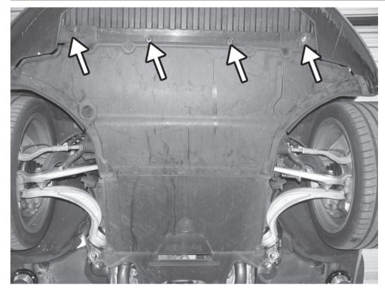
12) Remove the four T30 screws from the bottom of the front bumper cover.
