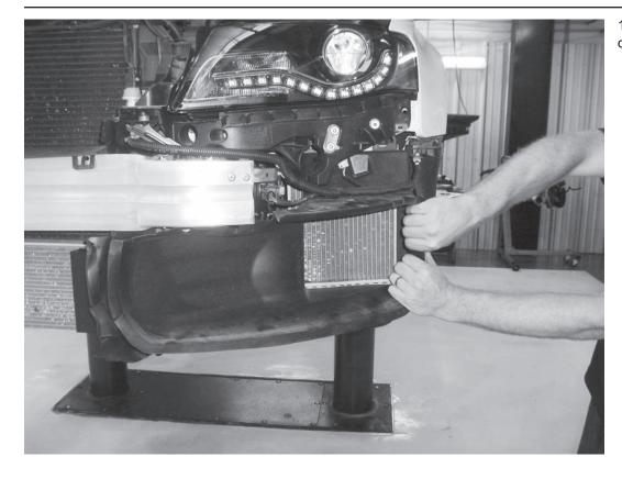
18) Carefully remove the radiator ducting, if equipped.
