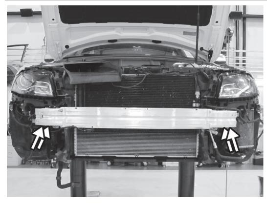
24) Unplug the horns and ambient air temperature sensor, unbolt the four 13mm bolts from the bumper beam, and remove bumper beam from the car. If equipped, disconnect and remove the headlight washer hose from inside the bumper beam.
