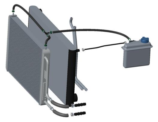
4) The later C7/C7.5 A6/A7 which have both engine coolant pipes facing the left side of the car can be configured as shown. The coolant tap is located between the factory coolant expansion bottle and the factory plastic bleed tubing. Both factory hoses to the APR CPS radiator will need to be extended with the supplied couplers, hose, and clamps.
