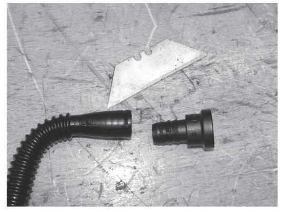
3) With a razor blade, carefully cut the plastic tubing off the fitting that was attached to the transmission and separate the fitting from the tube. The fitting will be reused.
