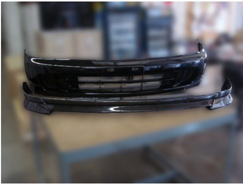
Fig. 1 Remove the bumper and place lip onto the bumper. Do not force the lip onto the bumper. Pay attention to the fitment to figure out what modification will be needed for installation.
