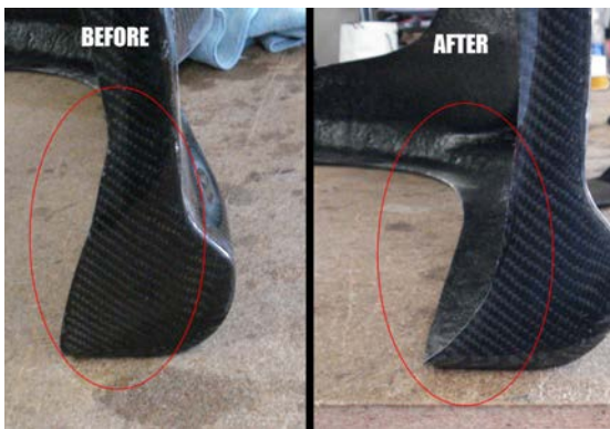
Fig. 3 Shaving and/or shaping might be required for proper fitment in various areas. Not all lips will require this step.
