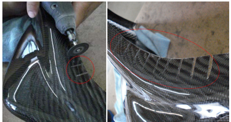
Fig. 4 Stress cuts can be used to relieve/prevent cracking during and/or after installation. Pictures above are an example of how the cuts can be made with dremel cutting wheel.
