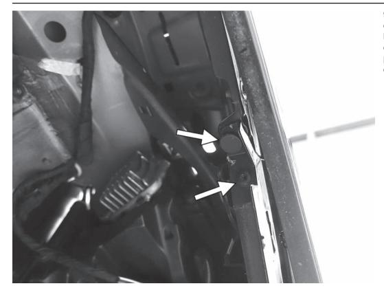
9) Remove the one push pin style connector and the one T25 screw holding the inside of the front bumper cover to the front fender. Repeat the previous steps on both sides of the car.
