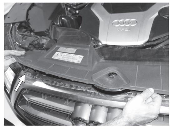
43) Replace the cover that connects the top of the bumper cover to the radiator support. Slide the back of the cover into the slot on the radiator support, and then press the front of the cover back into the tabs on the top of the bumper cover.
