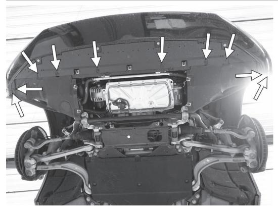
3) From the bottom of the front bumper cover, remove the four T30 screws along the front, the four T25 screws to the bottom of the wheel liners, and the two T20 screws on the bottom of the fender trim covers.
