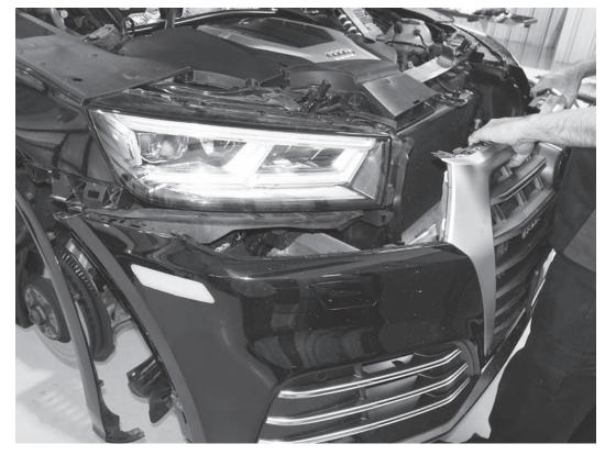
15) Lift the bumper cover and pull it forward to separate it from the car. Ensure there are no remaining connectors or lines holding the bumper cover to the car. Place the bumper cover aside, ensuring that the paint cannot get damaged.
