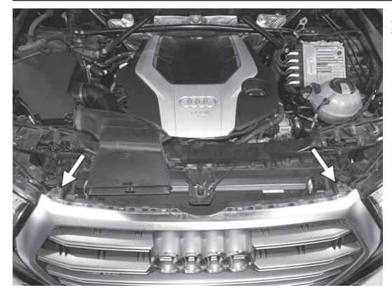
13) Remove the two T25 screws that hold the top corners of the grille to the radiator support.
