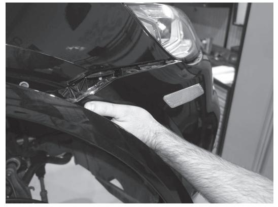
41) Place the both sides of the bumper cover back onto the mounting brackets located on each of the front fenders. Secure the sides by pressing the bumper cover into the mounting brackets.
