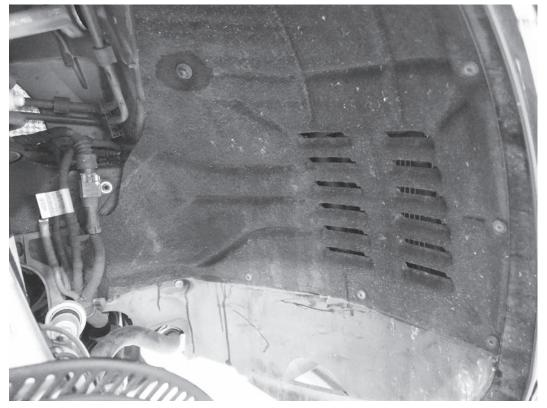
49) Place the wheel well liners back into their original locations. Reinstall the six T25 fasteners, four 10mm fasteners, and two push-pin style fasteners. Repeat the previous steps on the other side of the car.
