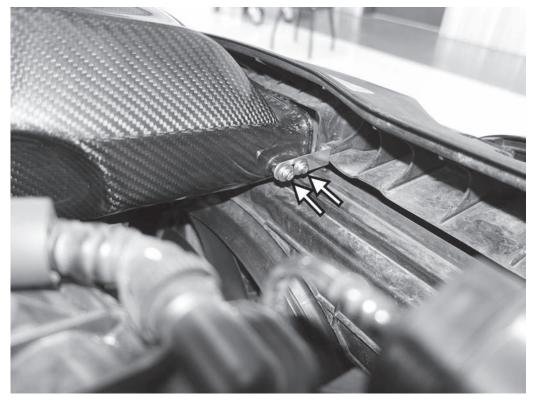
17) Using the supplied blue thread locker on the screws, install and tighten the two 3mm allen screws with washers to hold the front "L" bracket to the mounting boses on the front right of the APR intake.
