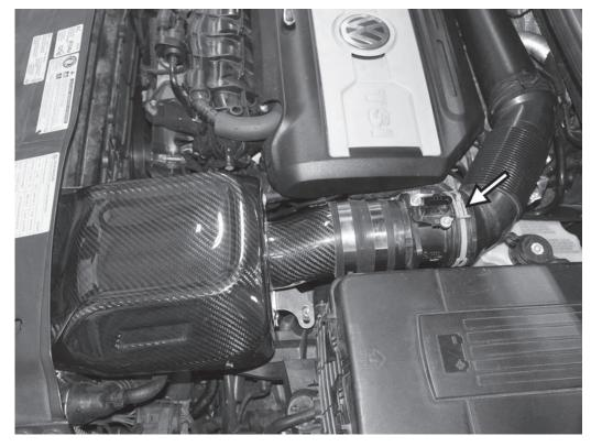
15) Loosely install the APR intake assembly in the car. Attach the according inlet elbow to the back of the MAF sensor housing and secure with the factory spring clamp.
