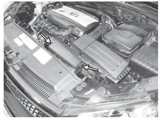
1) Lift up on the clips on both sides of the inlet scoop cover to remove the cover from the car.
