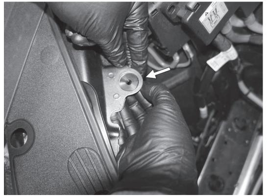
23) Locate the tab that has a round hole behind the right headlight. Install the APR airbox mount from underneath, allowing the adhesive to stick to the bottom of the tab.
