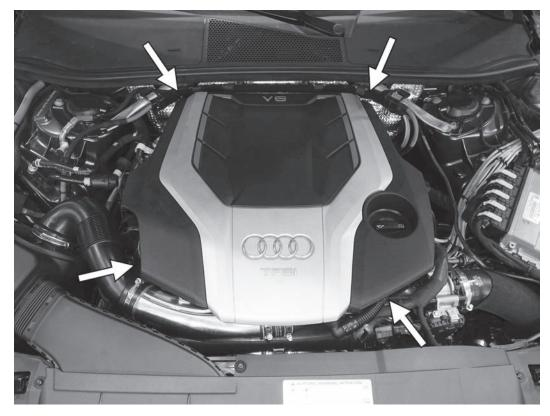
1) Raise the hood and remove the engine cover by lifting on each of the four corners of the cover.
