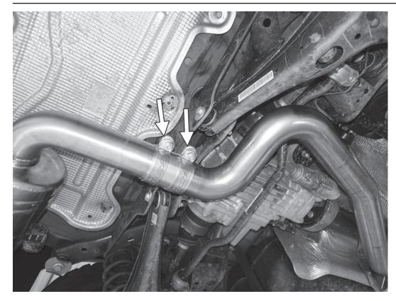
13) Connect the APR center section to the APR rear muffler with one of the supplied sleeve clamps. Slightly tighten the 15mm nuts on the APR clamp so the exhaust can still be manipulated, but do not fully tighten the nuts yet.
