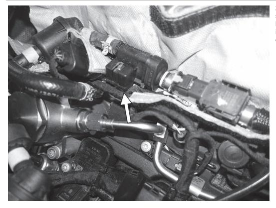
21) Loosely reinstall the flexible heat shield around the N80 valve assembly. Push the N80 valve back onto its mounting post on top of the right cylinder head.
