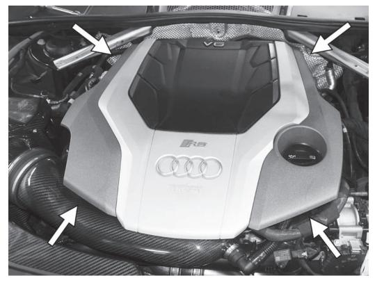
1) Raise the hood and remove the engine cover by pulling up on each of the four corners of the cover.
