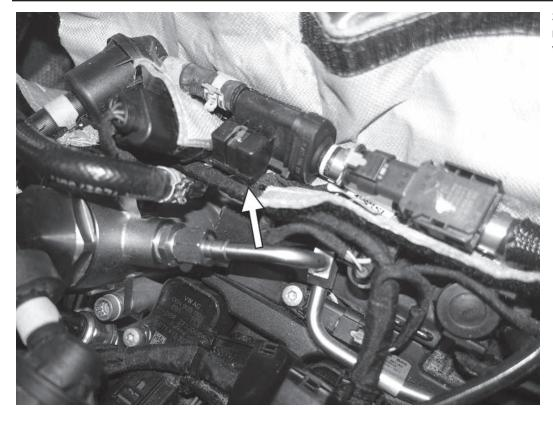
3) Carefully lift the N80 valve off its mounting location, and remove the flexible heat shielding from the car.
