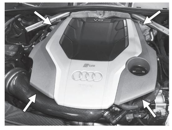
23) Reinstall the factory engine cover by pushing it down onto its four mounting posts.
