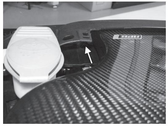
3) Remove the screw that holds the left side of the intake to the back of the radiator core support. Slide the intake out of the tab on the right hand side Separate the intake from the back of the core support.
