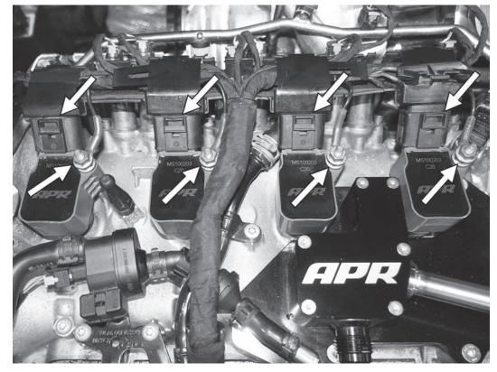
53) Flip the wiring harness from the front side of the engine over to the back side. Connect the four electrical connectors to the ignition coil packs. Install the ground wire for each coilpack onto the previously installed screw and place the 10mm nut onto the stud. While counterholding the 10mm screw with a wrench, tighten each 10mm nut to 9Nm (80in-lbs).
