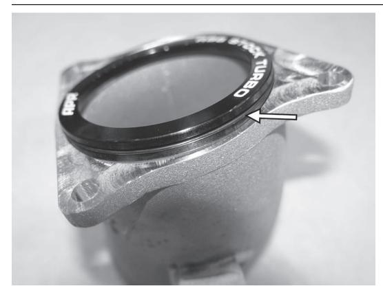
11) The turbo inlet adapters for the stock turbos are supplied with the intake kit. If using different turbos, contact APR for the correct adapters. Install the thin, supplied o-rings into the groove around the outside of the turbo inlet adapter rings. Then, place the rings into the cast turbo inlet pipes as shown.
