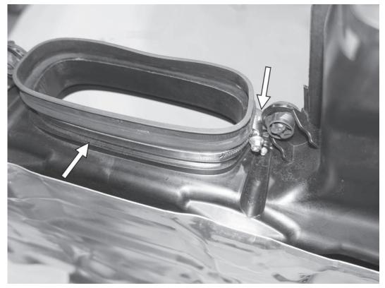
13) Install the APR airbox adapter onto the factory airbox. Loosely install the two factory T25 screws to hold the adapter in place. Make sure the bottom side of the supplied coupler is not pinched between the airbox and the adapter. Finally, adjust the hose clamp so it does not interfere with the airbox mounts, and then tighten the 7mm clamp to 5Nm (44in-lbs).
