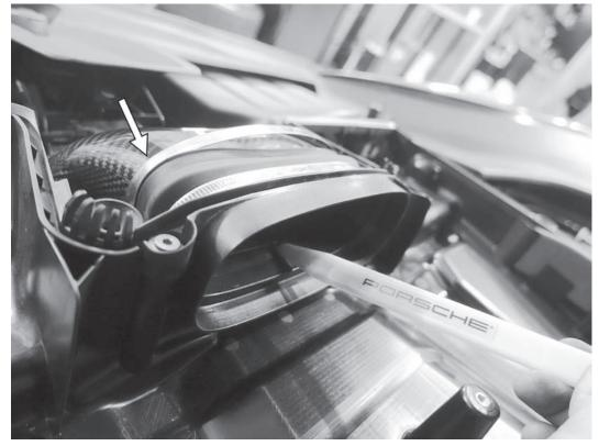
15) Place the remaining large hose clamp around the APR turbo inlet tube. Then place the factory airbox near the engine, sliding the rubber coupling from the APR adapter onto the APR turbo inlet tube. Use a plastic tool to work the rubber adapter around the outside of the APR turbo inlet tube.
