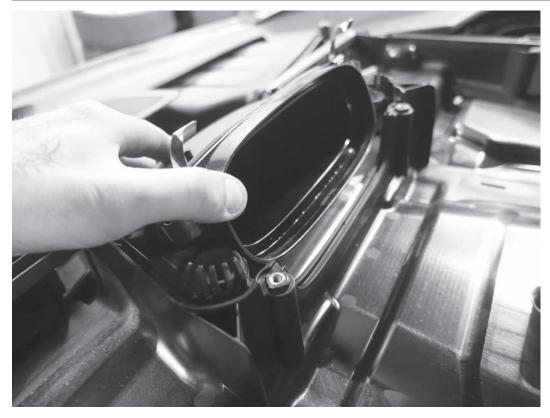
7) Lift up on the factory inlet tube to the turbo to separate the inlet tube from the airbox.
