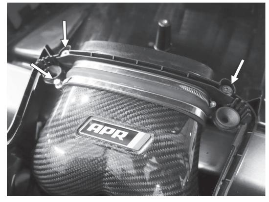
19) Install the 7mm hose clamp onto the front side of of the coupler, securing it to the APR turbo inlet tube. Tighten the clamp to 5Nm (44in-lbs). The install the two factory T25 screws, holding the APR airbox adapter to the airbox, and tighten the screws to 5Nm (44in-lbs).
