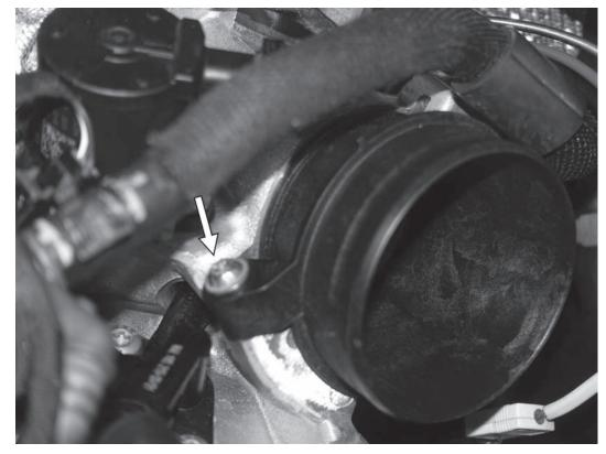
21) Once the tab on the APR inlet adapter is seated correctly, rotate the inlet adapter approximately 20° counter-clockwise until the mounting screw tab is aligned with the mounting screw hole on the turbo. Install the original T30 screw, and torque the screw to 9Nm (80in-lbs).
