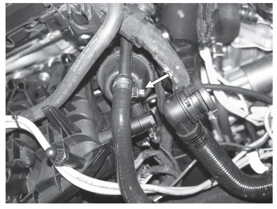
13) Remove the supplied cap from the metal pipe, and then install the APR coolant hose onto the coolant pipe by the intake manifold. Secure the hose with the supplied screw clamp.
