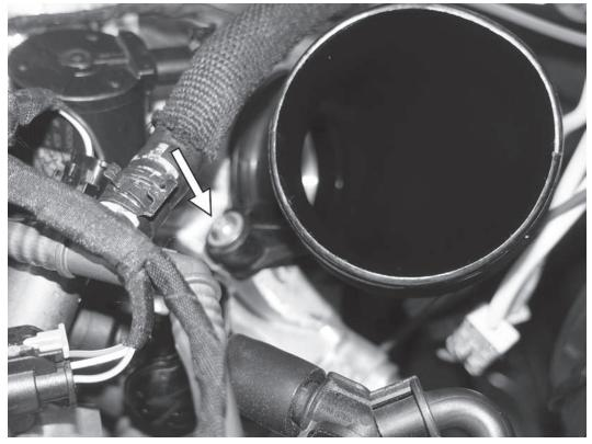
9) On the turbo inlet pipe, remove the T30 screw holding the inlet in place. Once removed, rotate the turbo inlet pipe clockwise, approximately 20°, to release it from the turbocharger.
