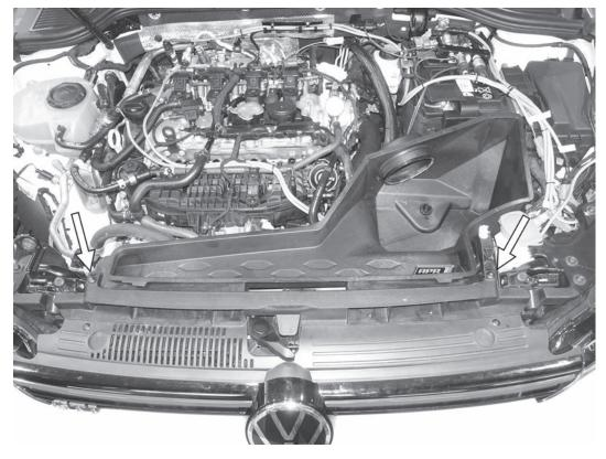
19) Install the two original T25 screws to secure the APR airbox base to the radiator core support. Tighten the screws to 2Nm (18in-lbs).
