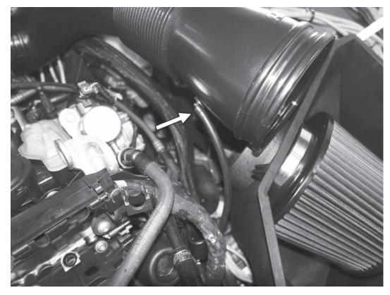
25) Install the previously attached rubber vacuum line onto the 90° barbed fitting on the side of the APR inlet pipe.
