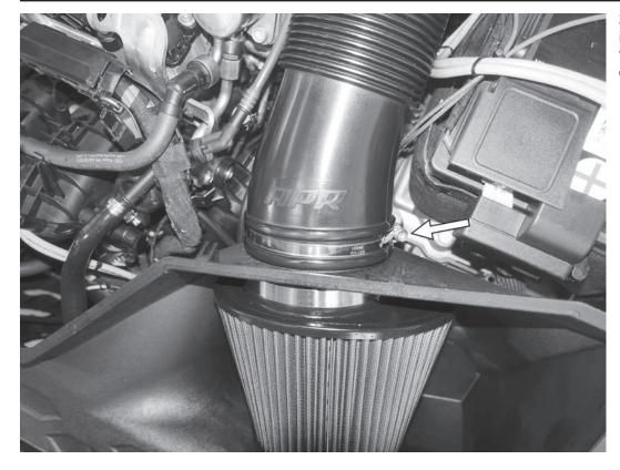
27) Place the other end of the APR inlet pipe on the flange on the back of the APR airbox. Secure both clamps on the APR airbox to 6Nm (53in-lbs).
