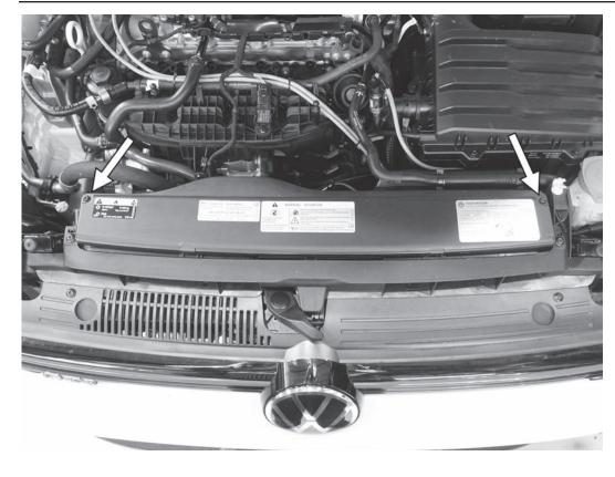
1) Raise the hood and remove the two T25 screws holding the airbox inlet cover.
