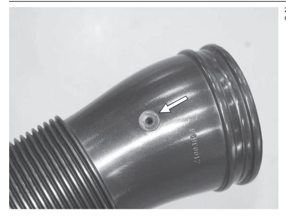
23) Install the supplied rubber grommet into the APR inlet pipe.
