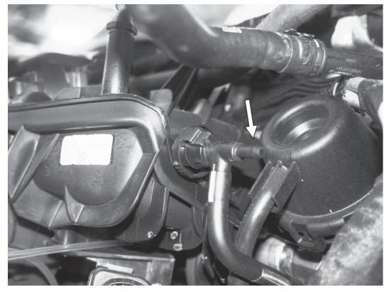
11) Follow the vacuum line that was previously attached to the airbox. Disconnect the line from the port on the side of the intake manifold. Install the supplied vacuum line to the solenoid.
