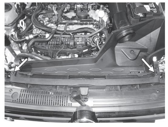
25) Install the two original T25 screws to secure the APR airbox base to the radiator core support. Tighten the screws to 2Nm (18in-lbs).
