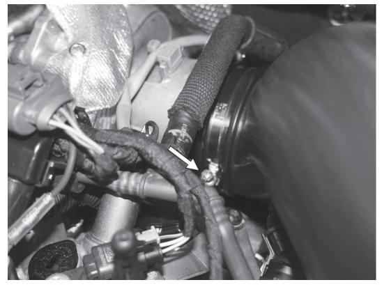
27) Once the airbox is in place, ensure there is no stress on the APR inlet pipe. Then secure the APR inlet pipe to the APR turbo inlet adapter by tightening the clamp to 6Nm (53 in-lbs).
