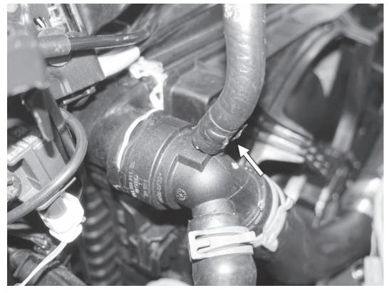
13) On the other end of the coolant line, remove the spring clamp and then hose from the top hose on the coolant coupling on the left side of the radiator. Use the supplied rubber cap to keep too much coolant from running out.
