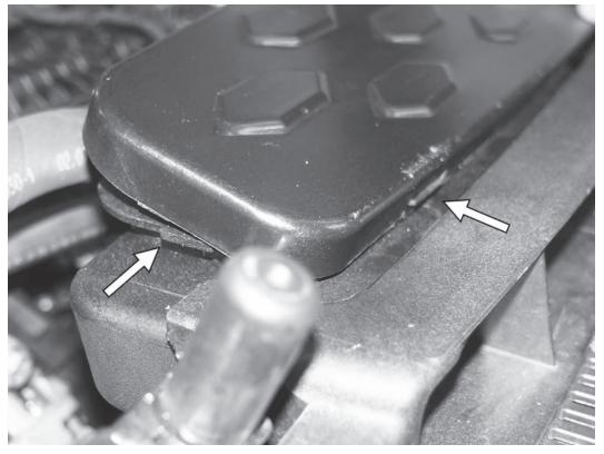
31) Install the airbox lid on the APR airbox by putting the front side of the cover on first. Ensure the two tabs on the front of the airbox go into the slots on the front of the airbox lid. Then, rotate the back of the airbox lid down. The lid will snap onto the tab on the right side of the APR airbox.
