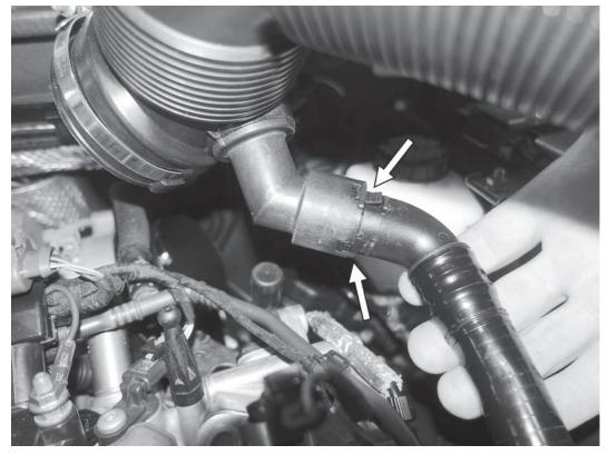
9) Disconnect the diverter valve pipe from the inlet pipe by squeezing on both sides of the connector on the diverter valve pipe and pulling it away from the inlet pipe.
