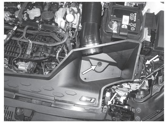
23) Place the APR airbox base in the car, pushing the installed grommets onto the factory airbox mounting posts. Loosely connect the APR inlet pipe to the flange on the back of the airbox. Make sure the sides of the APR airbox base aligns with the mounting tabs the factory airbox inlet base connected to the radiator core support. Ensure the APR airbox base is fully seated on the factory airbox mounting posts.
