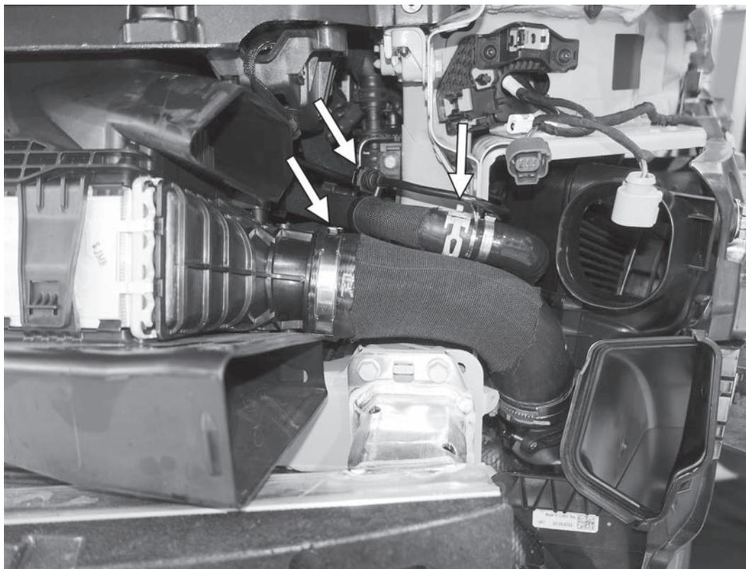
41) Reconnect the intercooler inlet hose to the intercooler and secure the stock clamp to 5.5Nm (49 in-lbs). Reconnect the vacuum line to the airbox at the factory coupler. Reconnect the diverter valve line to the APR coupler on the APR diverter valve hose and secure with the factory spring clamp. Repeat on the other side of the car.
