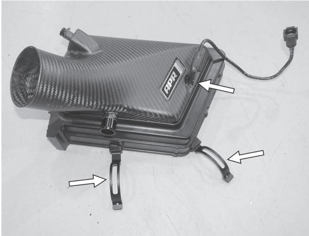
29) Install the factory vacuum line from the top of the airbox onto the APR airbox top in the same orientation. Install the supplied charge pipe brackets onto the APR airbox top as shown, with the longer bracket on the bottom and the shorter bracket on the side. Repeat on the other side of the car.
