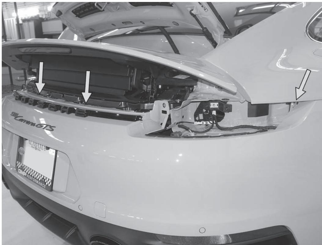
55) Reinstall the two remaining T30 screws to the top of the bumper cover. Tighten all two rear T30 screws to 3.2Nm (28in-lbs). Tighten the two previously installed outer T30 screws to 7Nm to (62 in-lbs).
