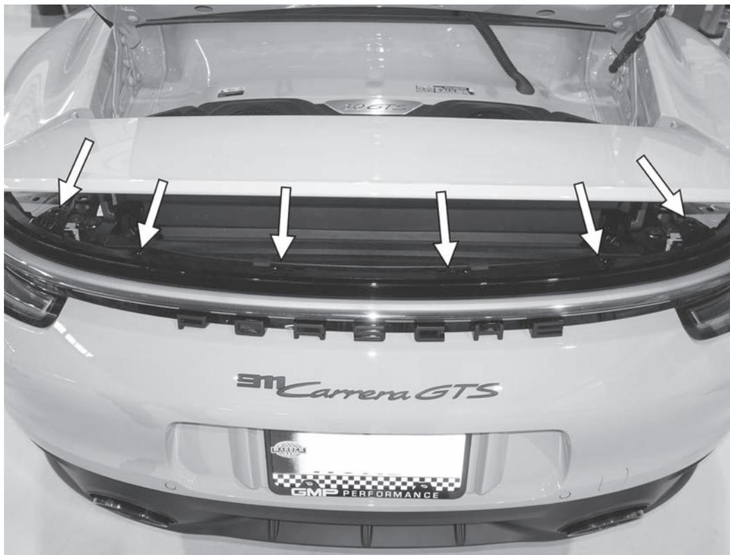
59) Secure the center taillight with the six T30 screws, and then tighten the screws to 6Nm (53 in-lbs).
