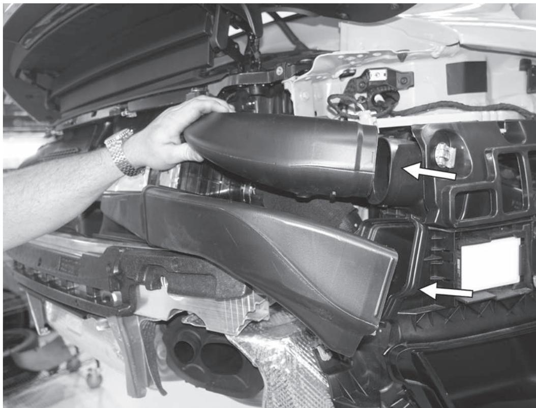
15) Pull off the two air guides, one for the airbox and one for the inter-cooler ducting. Separate from the airbox frame first, and then remove them from the car. Repeat on the other side of the car.
