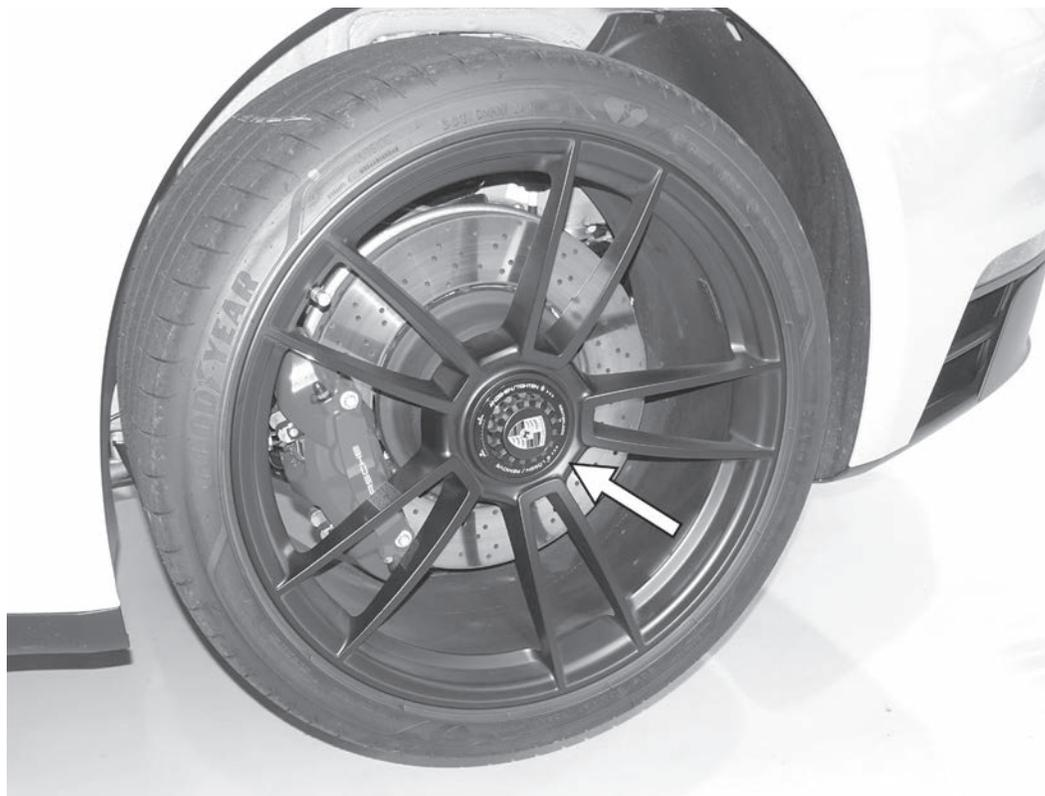
61) Reinstall both rear wheels and torque to spec, depending on the wheel type on the car. The rear spoiler can be lowered as well.
