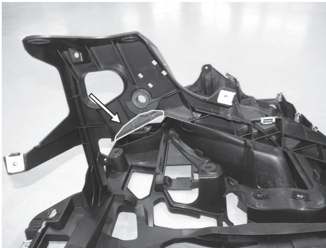
35) Depending on the style of rear bumper the car has, the airbox frame may be slightly different. If so, it may be necessary to slightly trim the frame by the side of the APR airbox outlet. This should involve removing around 15mm of the framework in the general area shown. Mount and dismount the APR airbox assembly as shown in the previous step and trim the airbox frame until there is sufficient clearance between the airbox frame and the airbox. Repeat on the other side of the car.
