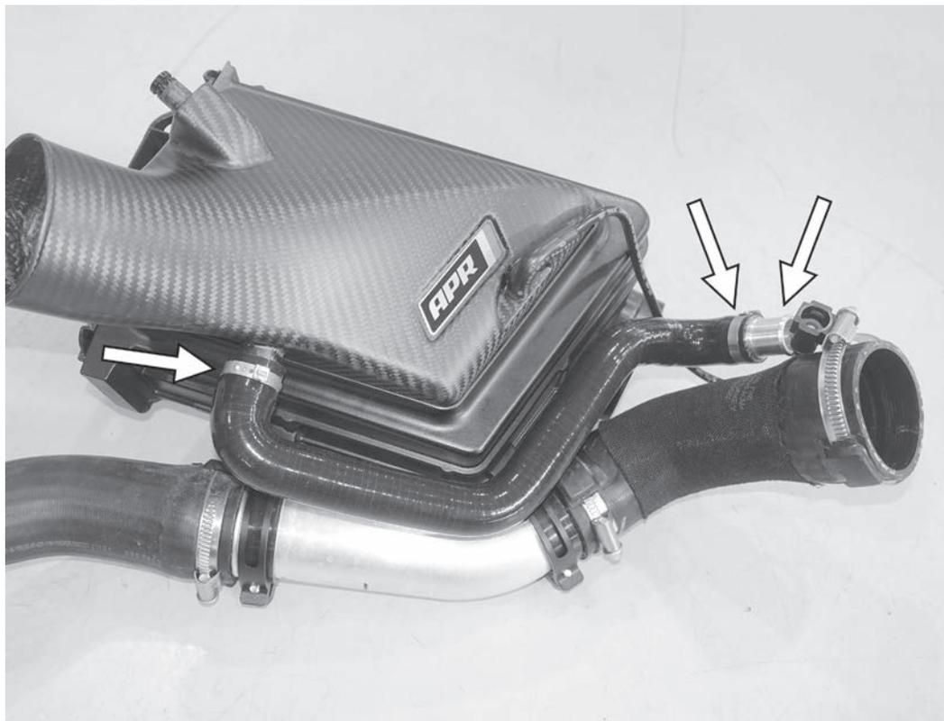
33) Install the APR silicone DV hose to the airbox with the supplied clamp, routing the hose as shown on the airbox. Install the supplied coupler on the other end of the DV hose, and secure with the other supplied clamp. Repeat on the other side of the car.
