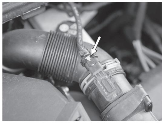
3) If equipped, disconnect the electrical connector to the MAF sensor. Slide the small white tab away from the sensor to unlock the connector, and then press down on the connector to release it from the sensor.
