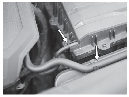
1) Disconnect the vacuum line from the side of the factory airbox. Lift the coolant hose out of the two clips on top of the factory airbox inlet.
