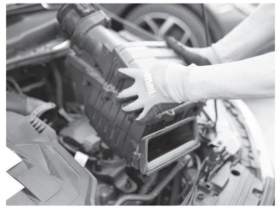
5) Lift the airbox assembly up and out of the car, separating it from the mounting posts underneath.
