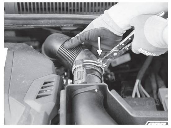
19) Reconnect the turbo inlet hose to the back of the MAF (or the APR MAF adapter) and secure with the factory spring clamp.
