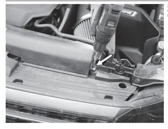
21) Reinstall the factory airbox inlet, securing it with the two original T25 screws.
