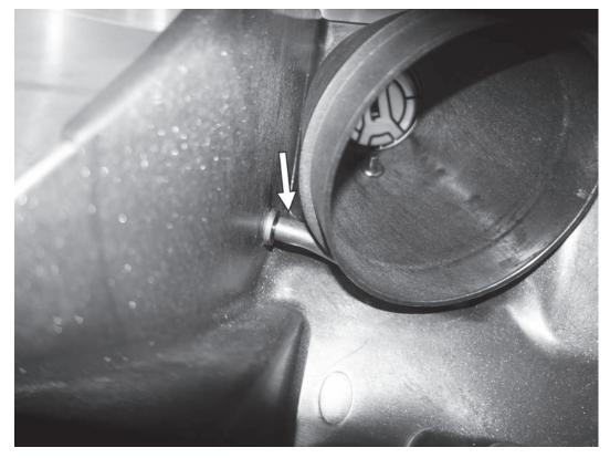
17) Connect the rubber hose from the APR filter adapter to the straight barbed fitting on the inside of the APR heat shield.
