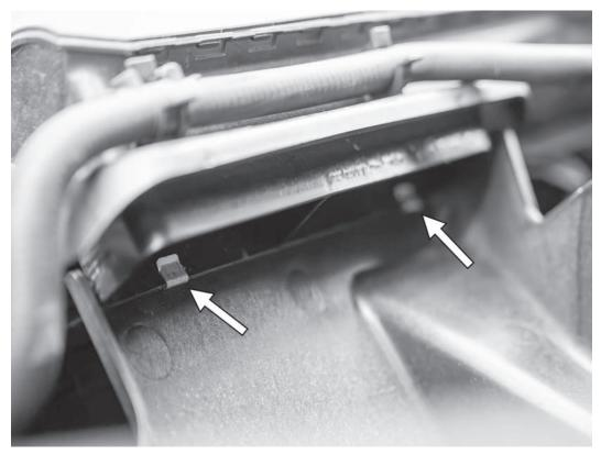
23) Connect the two metal clips on the front of the APR heat shield to the bottom of the factory airbox inlet. Again, some vehicles like the Tiguan, will not need these clips.
