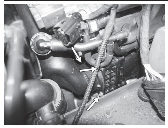
25) Unscrew the three T30 screws holding the charge pipe to the left intake manifold.
