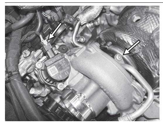
21) Disconnect the electrical connector on the diverter valve. Slide the grey locking tab back first, before squeezing the connector to unplug it. Remove the T30 screw from the oil feed line on the top of the turbocharger.
