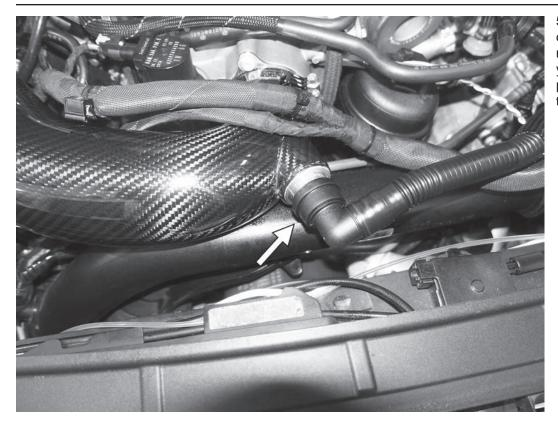
5) Use a 90° pick to loosen the PCV connection on the turbo inlet pipe near the front of the turbocharger. If you are reusing the same turbo inlet pipe on the APR turbo, you can leave this connection attached.
