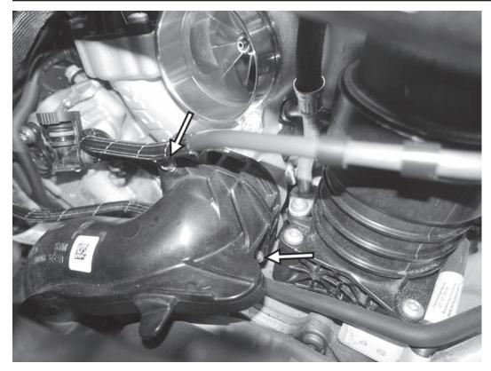
59) Replace the rubber gasket on the turbo outlet pipe with the new, supplied one, and then attach the turbo outlet pipe to the APR turbo. Tighten the two T30 screws to 9Nm.
