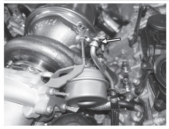
55) Remove the o-ring from the hard vacuum line and replace it with the supplied small black o-ring.
