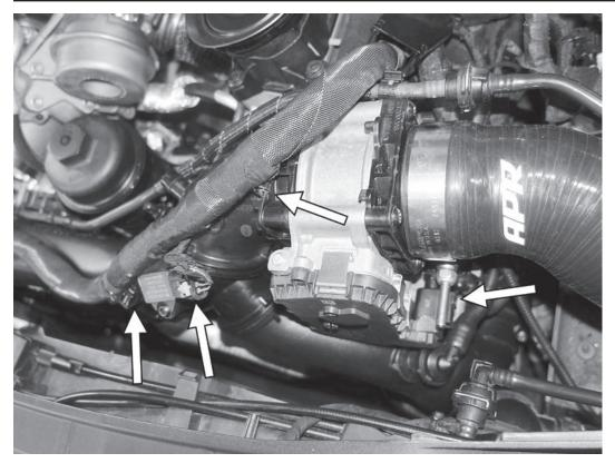
65) Reconnect the electrical connectors to the MAP sensor on the front charge pipe. Reconnect the electrical connector to the throttle boy. Reattach the two clips on the wiring harness their original mounting points on the front charge pipe.
