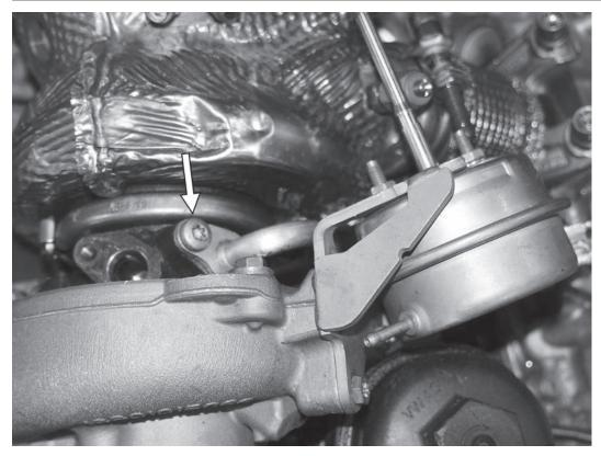
29) Remove the T30 screw from the coolant line on the top of the turbocharger and separate the line from the turbo.
