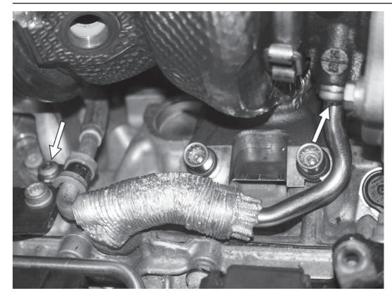
31) Remove the T30 screw from the coolant feed line on the right side of the turbo. Remove the T30 screw holding the coolant feed line to the right cylinder head, and then separate the coolant feed line from the turbo.
