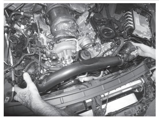
27) After ensuring everything is disconnected, carefully lift out and remove the front charge pipe from the car, with the throttle body attached. Depending on the options on the car, you may not be able to remove this pipe due to a wiring harness. If that is the case, leave the part in the car and it can be moved around for access to other components.
