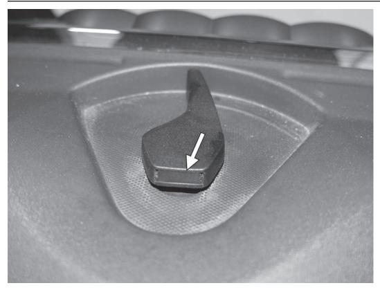
75) Reinstall the hood latch. The latch is keyed so that it can be only installed in one direction. Push the latch down until it clips fully onto the hood latch post.
