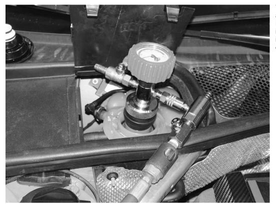
76) Refill the engine coolant using a vacuum bleeder style system. Follow the tool manufacturers instructions for vacuuming and refilling the engine coolant. Fill with new engine oil if the oil was drained.
