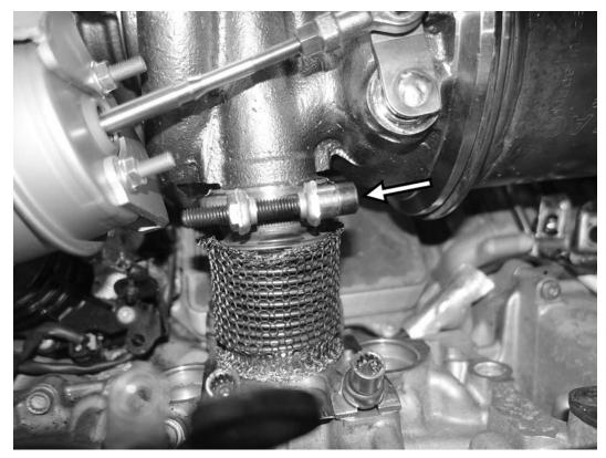
48) Once seated correctly, tighten the 10mm triple square on the exhaust coupler to 20Nm (177 in-lbs).
