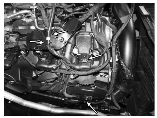
58) Reroute the oxygen sensor harness down the right side of the engine, reconnecting the harness to the clips on the side of the engine. Route the harness underneath the wiring harness as before, and then reconnect the oxygen sensor harness to the main harness. Reattach the electrical connector to the bracket on the side of the engine.
