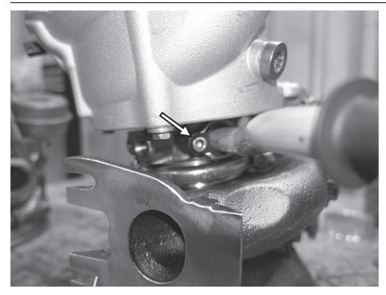
37) Lubricate both sides of the new, supplied oil drain line with clean engine oil. Install the oil drain line in the turbo with the previously removed factory plastic press-in plug. If the plastic plug breaks, a 5MM allen screw can be used to hold the oil drain line in place. This fastener is only used to hold the oil drain line in place while it is being installed, so it can be very lightly fastened.
