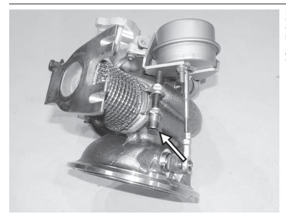
39) Install the exhaust coupler onto the APR turbo with the supplied v-band clamp, roughly orienting it as it was on the stock turbo. Tighten the 10mm triple square screw so that the exhaust coupler is still loose enough to be rotated, but not overly loose.
