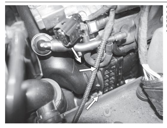
61) Loosely reinstall the three T30 screws that hold the front charge pipe to the left intake manifold. Try to rethread the screws in the original holes, as the self tapping screws can otherwise strip the intake manifolds.
