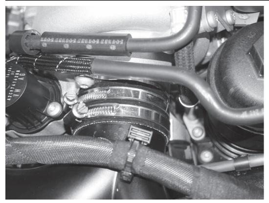
69) If using the APR intake, loosely reinstall the turbo inlet pipe with the silicone coupler and two clamps.
