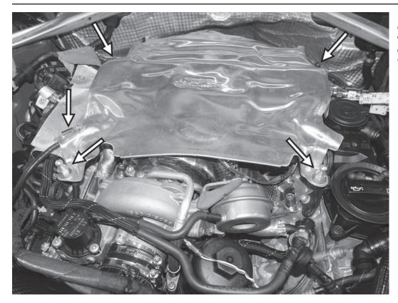
11) Remove the four 13mm engine cover mounting posts. Remove the wiring harness tab from the right side of the heat shield, and then remove the heat shield from the car.
