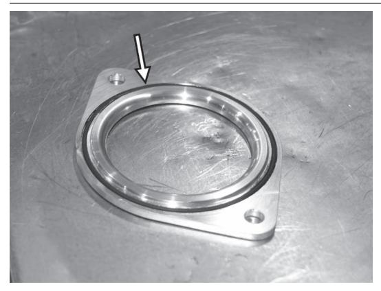
67) If installing the stock turbo inlet, install the supplied large, black o-ring into the groove on the back of the adapter for the turbo inlet. Use some silicone grease to hold the o-ring in place.
