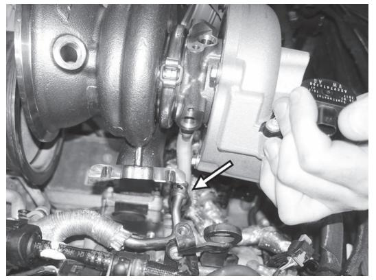
45) Place the APR turbo into the car, ensuring the oil drain line goes into its correct location on the engine. Lower the turbo so that oil drain line fits into the engine, while making sure the exhaust coupler on the left and the flange on the right side of the turbo correctly sit on the exhaust ports on the cylinder head.
