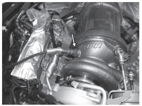
57) Install the oxygen sensor into the APR turbo, and tighten to 55Nm (40 ft-lbs).
