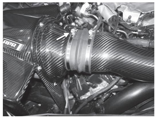
7) Loosen the turbo inlet pipe from the airbox and separate it carefully from the airbox.
