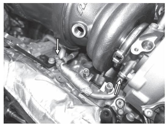
53) Replace the o-ring on the coolant line located on the right side of the engine with the last of the green o-rings, and then attach the coolant line to the turbo. Secure the line to the turbo and to the cylinder head with the correct T30 screws, and then tighten both to 9Nm (80 in-lbs).
