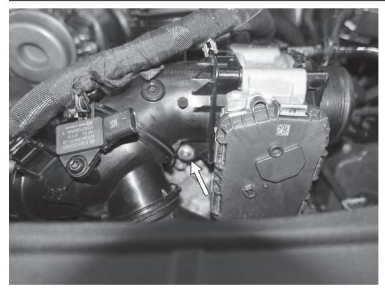
63) Reattach the front charge pipe to the engine by attaching the one T30 screw just behind the throttle body. Tighten the six T30 screws holding the front charge pipe to the intake manifolds to 6Nm (53 in-lbs) in a crossing pattern (top left, then top right, then inner on the left, outer on the right, then outer on the left, then inner on the right). Finally, tighten the T30 screw just to the right of the throttle body to 9Nm (80 in-lbs).
