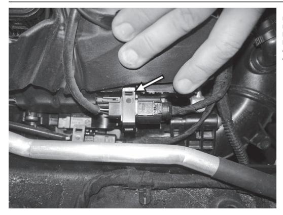
13) Unclip the oxygen sensor connector from the bracket, and disconnect the connector from the wiring harness. Route the oxygen sensor harness out from behind the ignition coil harness to completely free the oxygen sensor harness from the car.
