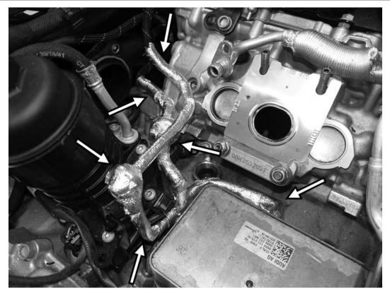
44) Using the supplied adhesive heat shielding, wrap the three vacuum lines with check valves in front of the oil cooler and behind the oil filter. Some lines can be wrapped by running the adhesive tape down the length of the hose and then wrapping it around, other areas will need to be spiral wrapped in the heat shielding. It may be necessary to clean these lines with a solvent first, like brake parts cleaner, in order for the adhesive to properly stick to the lines.
