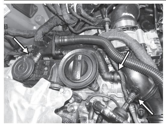
71) Connect the PCV hose assembly to the two connections on the PCV valve. If previously disconnected, reconnect the PCV hose assembly to the turbo inlet pipe as well. Reconnect the Norma style connection to the front charge pipe just behind the throttle body.
