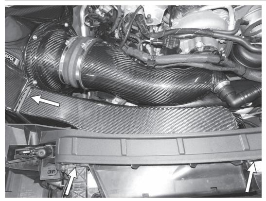
73) Replace the airbox inlet pipe and reattach it to the radiator core support with the two T25 screws.
