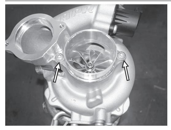
43) Install the supplied large black o-ring on the back of the billet APR turbo inlet flange, and then attach it to the turbo with the two supplied T30 screws. Tighten the screws to 9Nm (80 in-lbs). If installing the kit with the stock turbo inlet pipe, skip this step.
