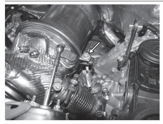
17) Loosen the 6mm allen screw (or T30 screw) on the v-band clamp holding the downpipe to the turbo. Once loose, pry up on the clamp and slide it to the back of the catalyst.
