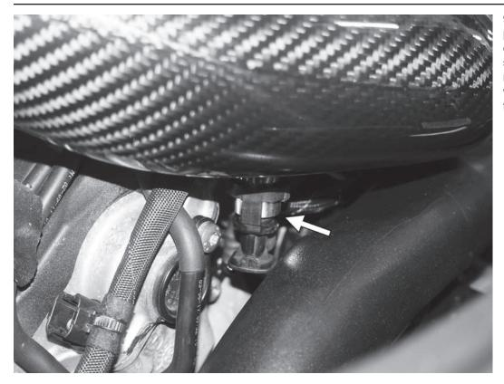
9) Slightly lift up on the turbo inlet pipe, and then disconnect the hose connection from the bottom of it by squeezing on both sides of the connector. Remove the turbo inlet pipe with silicone couplers and clamps from the car.
