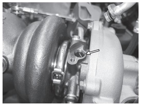
51) Pour a small capful of clean engine oil down into the hole for the oil feed line on the turbo.
