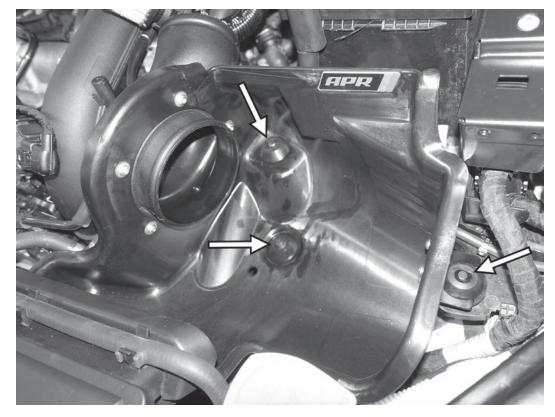
11) After making sure the front edge of the APR airbox is underneath the factory inlet guide, install the APR airbox onto the three posts the factory airbox sat on.
