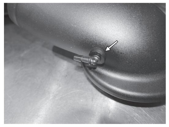
3) Using a lubricant, install the supplied rubber grommet into the side of the airbox outlet pipe. Install the 90° barbed fitting into the grommet as shown.
