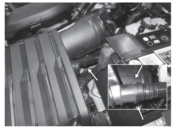
9) With the airbox slightly lifted, reach underneath the airbox outlet and disconnect the secondary air hose to the airbox. This is released by squeezing on both sides of the hose connection. Once released, lift and rotate the airbox out from the car.
