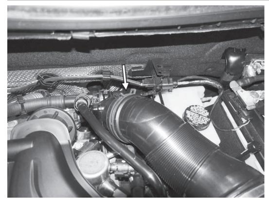
7) Squeeze the clamp on the other end of the accordian hose at the turbo, sliding it forward and off the connection to the turbo. Separate and remove the accordian tube from the car.
