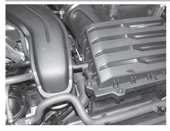
5) On the right side of the factory airbox, disconnect the vacuum line, leaving the rubber part of the line attached to the line, not the airbox.
