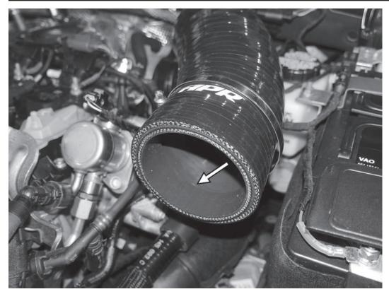
11) Loosely reinstall the APR silicone inlet tube onto the turbo inlet adapter. Depending on the airbox the inlet tube is being installed on, the supplied silicone inlet adapter may be needed. If so, install the silicone inlet adapter inside the inlet of the APR silicone inlet tube. The silicone inlet tube has a stop that will prevent the inlet adapter from going in too far. Loosely install the hose clamp over the inlet tube.
