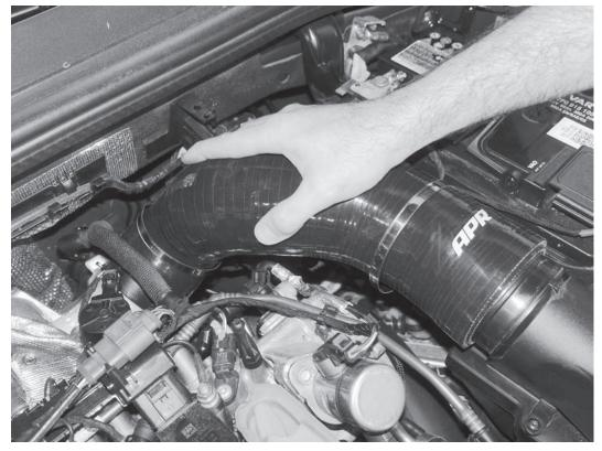
13) Install the APR silicone inlet tube onto the APR turbo inlet on the turbocharger. Ensure the silicone inlet fully fits on the turbo inlet all the way around (feel around on the bottom side of the hose to make sure it is fully seated).
