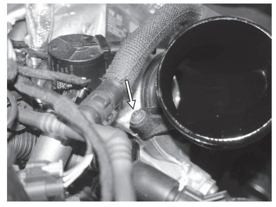
3) Loosen the T30 screw holding the factory turbo inlet to the turbocharger. Some oil in and around the turbo inlet is normal.
