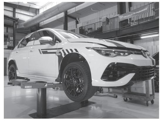
1) Securely place the vehicle on a lift or jack stands. While not required, it is a good time to do an engine oil service (leaving the new oil out of the engine until the installation is finished). The engine coolant can be drained. If you do not drain the coolant, some will be lost in the installation, but can be easily topped off after the installation. Also changing spark plugs would be advised, as you should have almost all the prerequised work performed.
