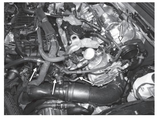
51) Reinstall the coolant vent line to the engine, being careful not to bend the line. Reconnect the two tee fittings behind the number four cylinder and one in front of the high pressure fuel pump. Reconnect the hard coolant line from the coolant hose that runs by the factory airbox. Finally, install the T30 screw by the charge pipe mounting point and tighten to 9Nm (80 in-lbs).
