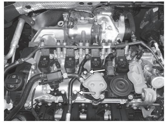
53) Reinstall the ignition coilpacks in the engine, but do not secure them. Reinstall the two T30 screws holding the turbo coolant return line to the top of the valve cover. Tighten both screws to 8Nm (70 in-lbs).
