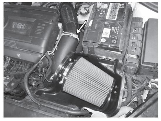
15) Reattach the factory intake tube to the back of the APR intake, and secure with the factory spring clamp.
